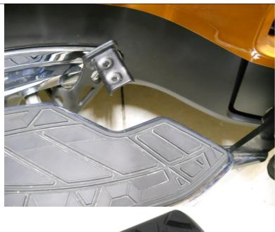
Remove your stock rubber pad by removing the 2 screws in the bottom of it.
