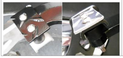
The Extension can be installed above or below the original brake pedal using the supplied cover pad, spacers and hardware, depending on desired height and floorboard configuration. You can also opt to not use the spacers on top if it works better for your desired height.
