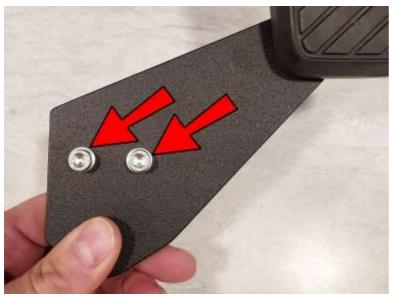
Place the other two bolts into the lower holes of the BPE4.
