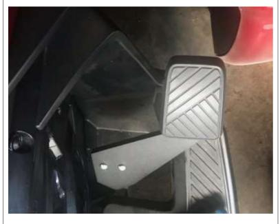
Place onto the stock brake pedal and secure with the other M6 Washers and M6 Nuts.
