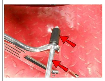
Insert an M10-1.5 x 170mm Bolt into the top hole of the Plate then place a 2.8" Spacer on the bolt.
