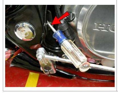
Push the Brake Pedal forward and remove the screwdriver. The Brake Pedal should rest tightly against the foot peg clevis.
