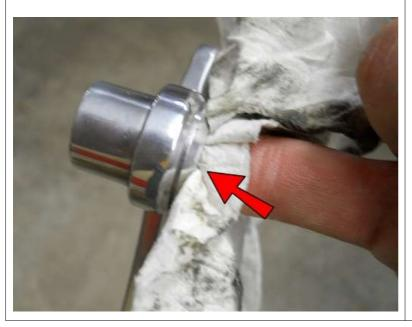
The inside of the Brake and Shifter Pedals will likely have some polishing compound residue. Use a cloth or paper towel and make sure the inside is ABSOLUTELY clean. This can affect how well your Pedals will rotate.
