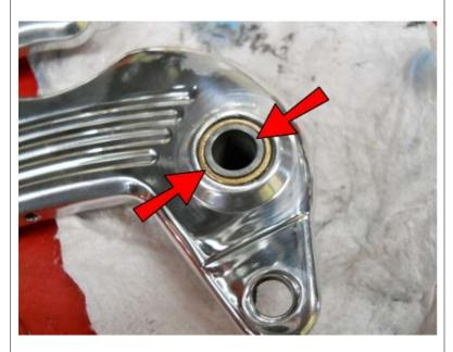
Place a SLV1 into the 5/8x1/2 Bronze Sleeves and insert them into the Brake and Shifter Pedals.
