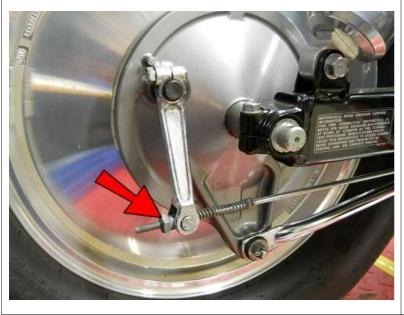
Adjust the brakes by going to the rear of the bike, and tighten or loosen the brake rod adjusting nut if needed. You want enough tension to allow a small, comfortable amount of movement to actuate the brake but do not over tighten, as this will keep the brakes from releasing fully.
