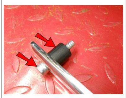
Insert an M8-1.25 x 60mm bolt into the rear slot of the Brake Side Plate then place a 1.5" Spacer on the bolt.
