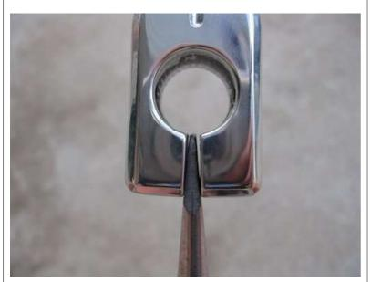
Hold the brake arm firmly and insert a large flat head screw driver or better yet, a small chisel, into the end of the Brake Arm and carefully tap the handle on a hard surface to spread the spline opening apart. The goal here is to spread the hole just far enough apart to easily slide the Brake Arm onto the brake spline. Note: This can be easy OR the most frustrating part of the install if the hole is not spread apart enough, (but only just enough, not too much).
