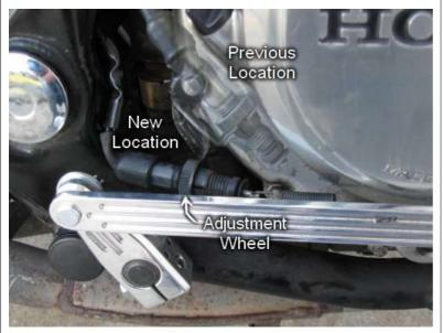
Remove the case bolt shown as "previous location" and remove the hose stay if it has one. Place that bolt into the small hole in the new Brake Switch Mount and insert your brake switch into the larger hole in the brake switch mount then replace this assembly into the case making sure to align in a straight line of movement for the spring. Note: This picture is from a V45 and will differ slightly.
