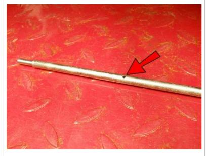
Orient the Brake Linkage with this small hole toward the rear of the bike.
