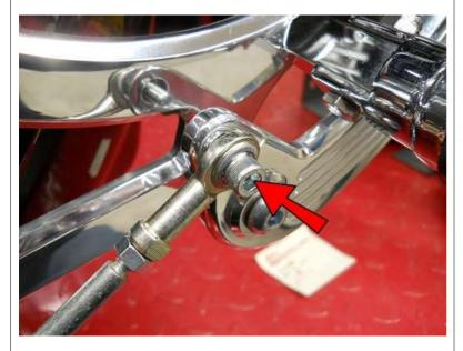
Place the Linkage on the Brake Pedal and insert an M6-1.0x25 Bolt.
