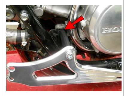
Insert into the motor mount hole and secure with an m10 Nut, then go back and tighten the 3 rear M8 Bolts.
