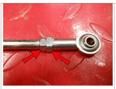
Thread an M6 Nut and M6 Spherical Rod End all of the way onto one end of the linkage and the M6 Left Hand Nut and M6 Left Hand Spherical Rod end all of the way onto the other end.
