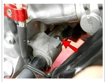
Now secure the M10 Bolt with a 3/8" Zinc Washer and an M10 Nut on the back side of the motor mount.
