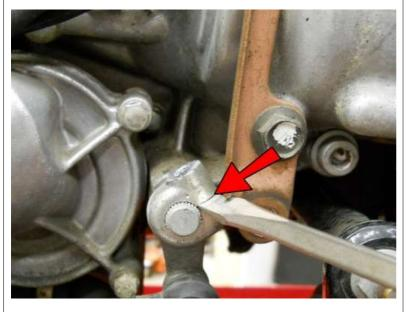
Using a screwdriver to help loosen the shifter arm, slide it carefully off of the spline, noting the position of the tiny alignment marks.
