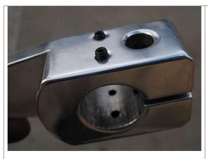
Start the 4 Set Screws into the Brake Arm but assure they do not protrude through the inside.
