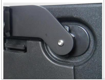
Attach using the original threaded hole and the supplied bolts.
