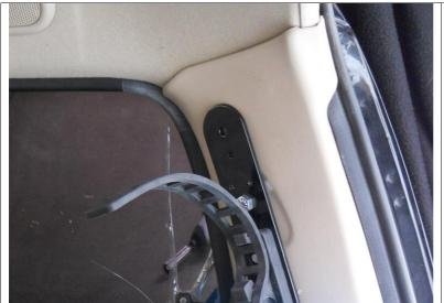
Remove the rear seat belt and secure the mount to the D pillar.
