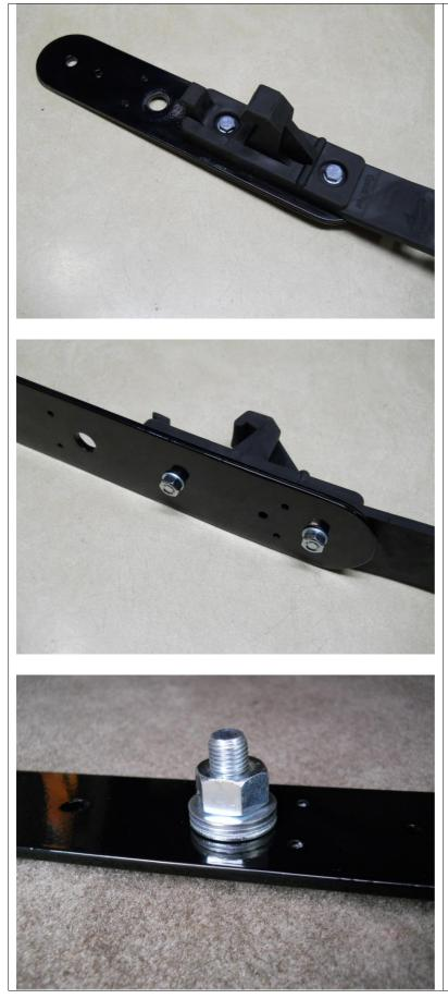
Place the Quick Fist Longarm onto the mount as shown and insert M6 bolts into washers and into the mount.
