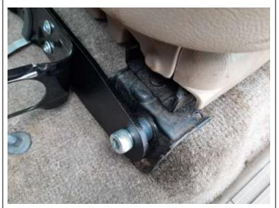
Move the seat all of the way back to access the seats front bolts and remove the plastic cover over the bolts, then remove the bolts.
