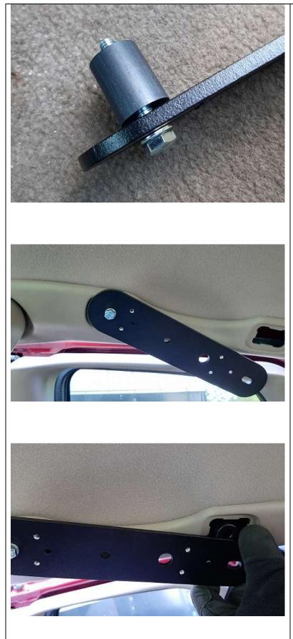
Place the short bolt into the end of the mount with the round hole (not the slotted end) and place the short spacer onto the back side.
