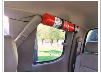
Attach the fire extinguisher bracket to the mount with the small screws. Put the curved end of the fire extinguisher bracket (that holds the nozzle end) toward the back of the truck. Note: A thread lock compound such as Loctite is a fantastic idea here.
