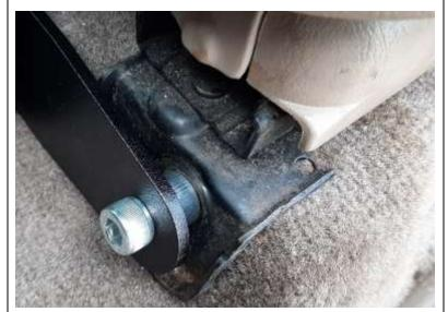
Move the seat all of the way back to access the seats front bolts and remove the plastic cover over the bolts, then remove the bolts.
