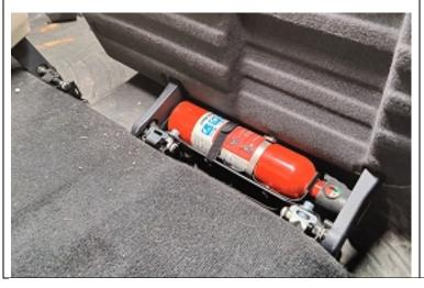
Most extinguishers will allow the seats to be folded all the way up. The seat may hit the nozzle or the body but only so slightly that it will not be a problem.
