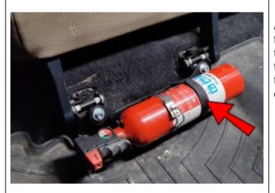
All extinguishers are sized slightly different. I find that adding a Velcro cinch strap helps keep things tight if the extinguisher is a little skinny for the clamp. It is also very helpful in keeping the extinguisher secure if the clamp gets kicked open.
