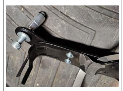
Insert the supplied bolts into a washer, then into the FM20. Now slide one of the short spacers and one of the longer spacers onto the bolt as shown. Do this on both ends of the FM20.
