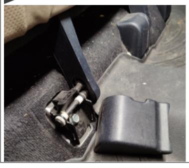
Remove the plastic covers over the seat mounts. They easily pop off with a flat heat screwdriver.
