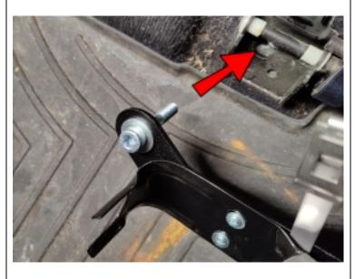
Secure the new bolts back into the seat mount holes and tighten. Note: You might have to lift the seat a little to line the holes back up.
