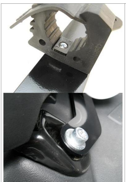
Insert small screws into the countersunk hole in the black plastic square washers.
