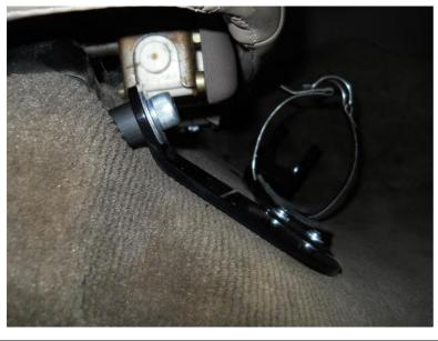
Place the spacers under the mount and secure with the large bolts and washers as shown.
