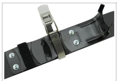
Attach the fire extinguisher bracket to the mount with the supplied small screws, washers and nuts. Depending on which side you are installing the mount on, put the curved end of the fire extinguisher bracket (that holds the sprayer end) toward the CENTER of the vehicle.
