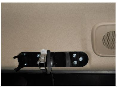
Use the other washers and small screws to attach the fire extinguisher bracket to the mount as shown.
