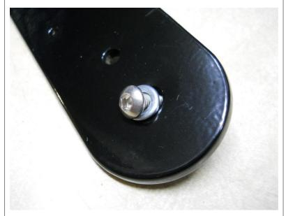
Insert the supplied long screws into the washers, then into the end holes of the mount.
