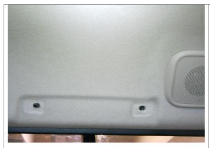
Attach the mount to the existing holes in the ceiling. Align the mount so that the LARGE hole in the center of the mount is more toward the FRONT of the vehicle.
