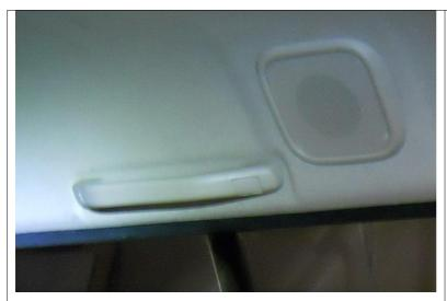
To remove the handle, pry out the square plastic screw covers with a small screwdriver and remove the screws.
