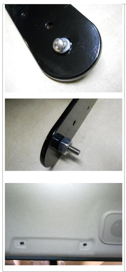
Insert the M6 screws into the washers, then into the end holes of the mount.
