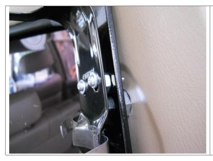
Using the other nuts supplied as spacers on the 4 screws as shown, attach the fire extinguisher bracket with the curved end up.
