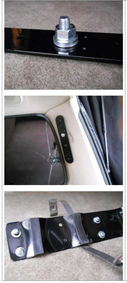
Place the supplied large bolt into the mount, then place 3 washers and the large nut onto the back side as shown. The nut does nut thread onto the bolt, it is just being used as a spacer.
