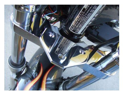
Remove the front bezel and bulb from the replacement headlight. Run the headlight wires into the small hole in the replacement headlight shell and then install onto the HM1 leaving bolt hand tight for now.
