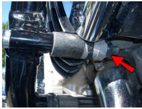
Secure with the nut (supplied) and tighten this bolt and the front bolt.
