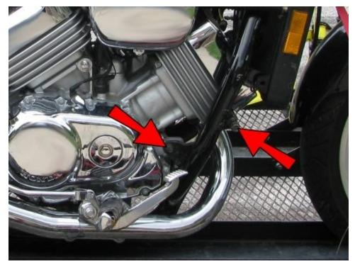
Remove these two motor mount bolts. The bolt that you remove from the front will now be used as the rear. The bolt and nut (supplied) will now be used on the front.
