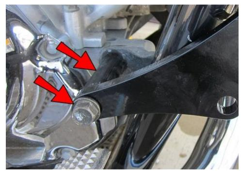
Loosely thread in the rear bolt using the long spacer (supplied).
