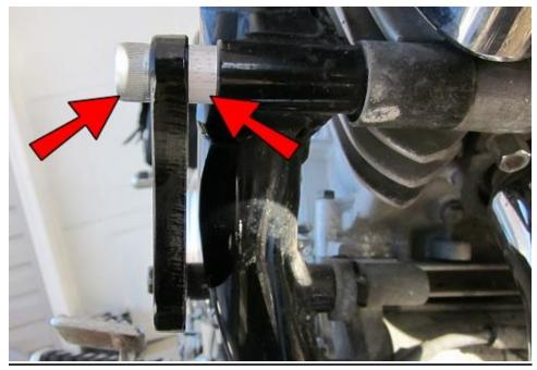
Insert the long bolt (supplied) into the front and use the short spacer (supplied) between the HPM2 and the frame and keep the stock spacer between the frame and the motor in the same place as it was.
