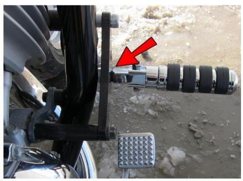
Attach a foot peg to the HPM2, tighten and repeat on the other side.
