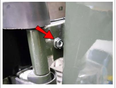
Apply some thread lock to the M6-1.0x30 Screw previously inserted and secure with an M6 Washer and Nut. (This is most easily done with the door open, standing on the bumper and wrenching from above.)
