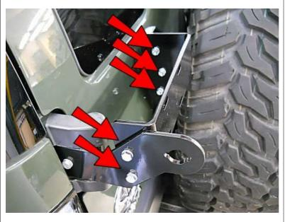
Now secure the Hanger Bracket with M6 Washers and Nuts on all 5 screws and tighten. (OK, yes it's a spare, no, yours should NOT be on yet.)
