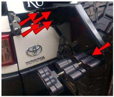
Using the last of the M6 Screws, Washers and nuts attach the RP2 Bracket to the Hanger and only finger tighten at this time. Unless you have very large tires you should be able to slide it all the way to the right of the slots in the Hanger.
