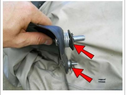
On the other two M10 Screws on the right side of the spare tire carrier, place THREE 3/8" Zinc Washers and one of the rubber washers removed earlier onto each one.
