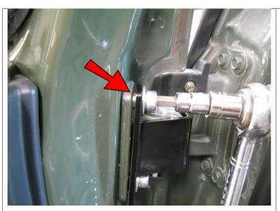
Line up the holes of the Left Bracket to the hinge and use the M10 Screws with Washers and Alignment Sleeves to connect the Bracket. Make sure the Alignment Sleeves go into the alignment holes on the Left Bracket AND the hinge. Do NOT tighten yet.
