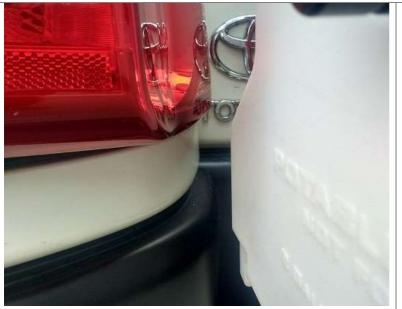
Mount your RotoPax Cans and then SLOWLY open the door to check for clearance. Make sure there is enough room to allow the door to open at a normal rate without hitting your taillight hard enough to damage it.
