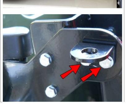
If you are installing the Optional CB Antenna Mount, use the supplied M6-1.0x20 Hex Head Cap Screws, M6 Washers and M6 Nuts to secure as shown, then install your antenna.
