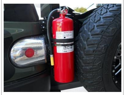
Temporarily mount your cylinder and then SLOWLY open the door to check for clearance. Make sure the cylinder does NOT touch the taillight lens and that the Main Bracket does not touch the black plastic molding under the taillight.
