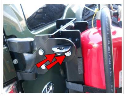
If you are installing the Optional CB Antenna Mount, use the supplied M6-1.0x20 Hex Head Cap Screws, M6 Washers and M6 Nuts to secure as shown.
