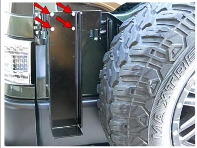
Using the last of the M6 Screws, Washers and nuts attach the Main Bracket to the Hanger and only finger tighten at this time. Unless you have very large tires you should be able to slide it all the way to the right of the adjusting slots in the Hanger.
