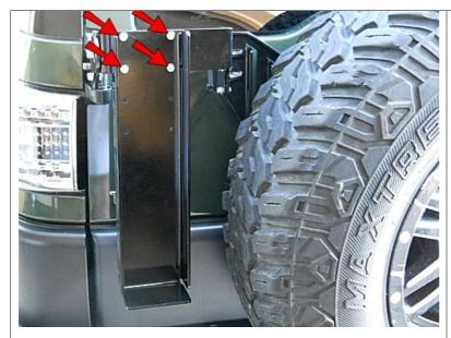
Once you have checked that your clearance is all ok, remove the cylinder and tighten these screws.
