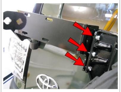
Place the Hanger Bracket between the Left and Right Brackets as shown and insert three M6 Screws and Washers here. (No, you do not see a spare tire already mounted. That is an illusion)
