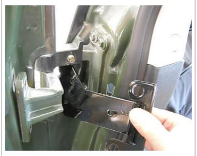
Insert the Left Bracket through the hinge as shown. If you tilt it at the correct angle it will go easily, don't force it, just try another angle if it isn't going.
