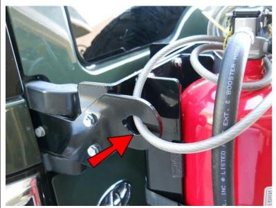
If you are NOT installing the Optional CB Antenna Mount, this hole can be used as a lock-down point to secure your cylinder.
