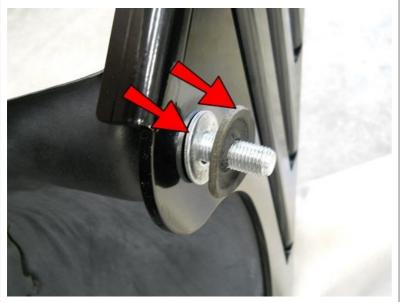
Place a 3/8" Zinc Washer and one of the rubber washers removed earlier onto the back side of those two M10 Screws. Later models had a thin stick on plastic washer instead of the nice thick rubber ones. If your washers are not reusable you can get the stick on ones from Toyota, Part #51998-35020 or you can wrap some electrical tape around the Zinc Washer to protect the paint.
