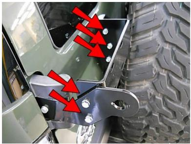
Now secure the Hanger Bracket with M6 Washers and Nuts on all 5 screws and tighten. (OK, yes it's a spare, no yours should NOT be on yet.)
