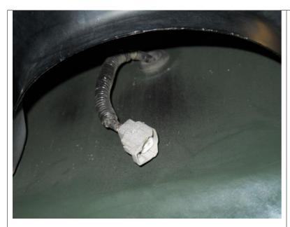
Remove your spare tire, cover and camera if applicable and disconnect the camera wire from the spare mount if there is one connected to it.
