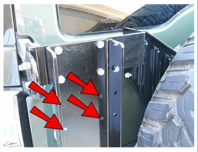
For larger cylinders and/or larger tires, you might need to mount the Main Bracket in a higher position using the other holes. This will create better clearance as well as distribute the weight more evenly top to bottom for increased strength and less vibration.
