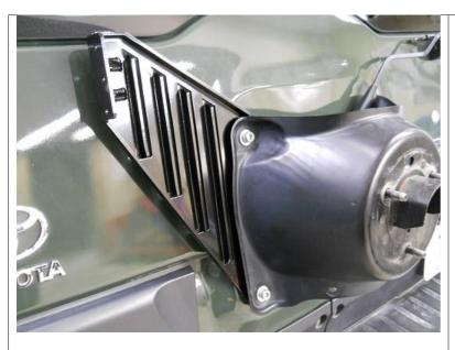
Being careful not to let the carrier or the Right Bracket touch the paint, thread all 4 Screws into the carrier mounting holes on the door. Thread them most of the way, but leave them loose enough that you can move the Right Bracket up and down.
