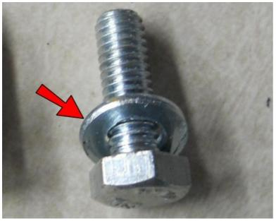
Place M6 Washers onto all 9 of the M6-1.0x18 Hex Head Cap Screws.
