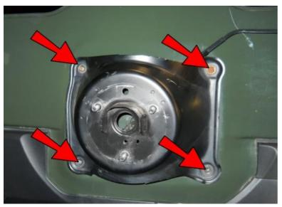
Remove the two bolts and the two nuts holding the spare tire carrier to your door. When you remove the carrier, there will be 4 rubber washers on the bolts or stuck to the paint surface. Carefully peel them off, you will re-use them.
