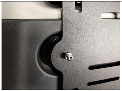
Slide the Panel over the bag hanger and line up the hole in the Panel with the center of the Spacer. Start the thread of an M6-1.0x45 BHCS in the hole a few turns.
