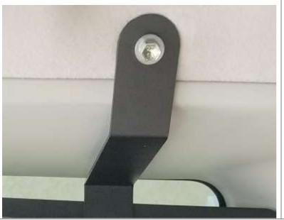
Using the bolt previously removed from the hanger hook, snug the top of the Top Mount against the ceiling.
