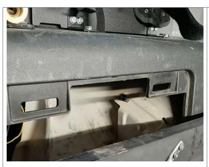
Open the access panel and secure the Bottom Mount Bolts first with a 1/4"x1.5" Washer, then an M6 Washer and an M6 Nut and tighten.
