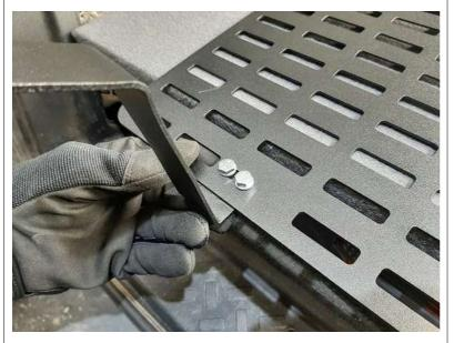
Attach the Top Mount to the BACK of the Panel using the M6 Hex Bolts and secure with another Washer and M6 Nut on the back BUT only finger tighten at this point. Keep them loose enough that the mount is still able to move.
