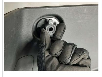
Insert the supplied spacers into the bag hangers. (If they do not go in all the way flush, they will when you tighten things up.)
