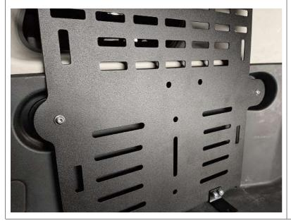
Now tighten the bolts just enough that the Spacers seat and the Panel rests where it will end up when complete.
