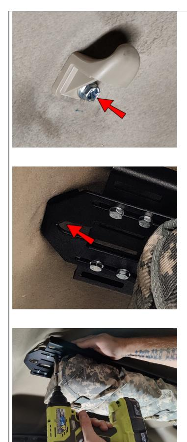
Open the cover and remove the hooks from the ceiling of the cargo area. You will use the bolts removed, in the next step.
