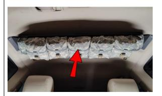
Remove the handles from the ceiling of the cargo area. You will use the bolts removed, in the next step.
