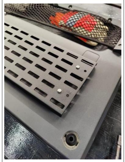
Replace the Molle panel and attach it to the door panel with the five M6-1.0x45 BHCS. They will thread into the slightly smaller holes you drilled.
