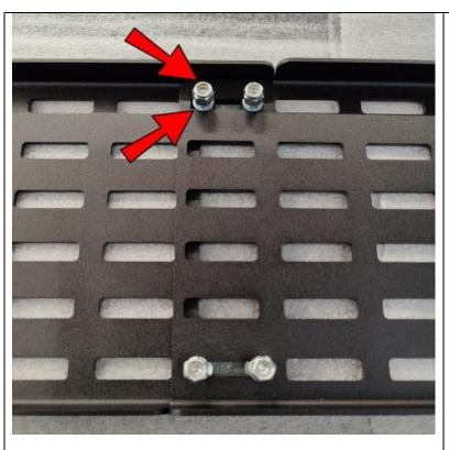
Place the other panel on top of the bolts and put a Washer and a 1/4-20 Locknut onto each Bolt and tighten all four Bolts.
