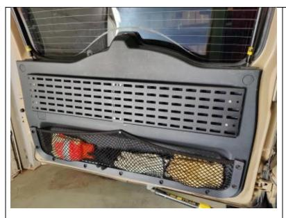
Re-attach the door panel by snapping it back into place and replacing the bolts and covers at the top.
