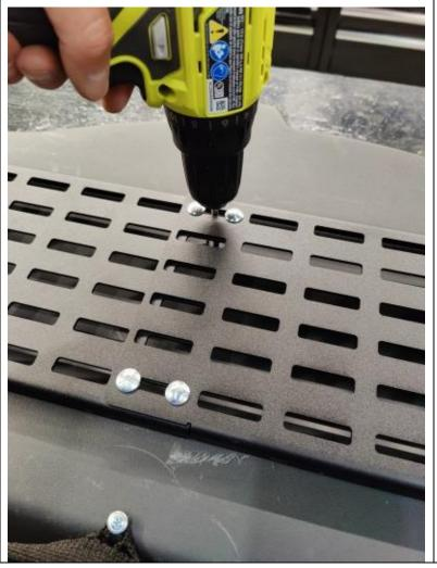
Also, drill a 7/32" hole at the TOP ONLY of the center of the Molle panel, right between the carriage bolts.
