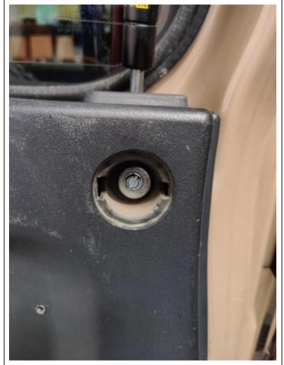
Remove the covers over the 2 bolts that hold the door panel on. Remove the bolts. Pop the panel loose from the door. Open the rear window. Remove the panel from the door.
