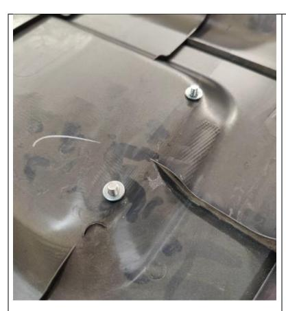
Carefully flip the door panel over and place M6 Washers on the Bolts.
