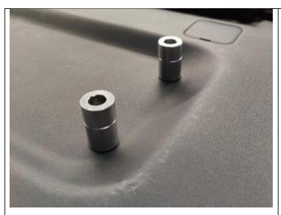
Remove the Molle panel and stack ONE of the .5" Spacers and ONE of the .75" Spacers onto each other, on each of the 5 holes you drilled.
