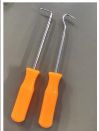
Pro tip: You can buy a set of these brake picks for a couple bucks at Harbor Freight. They are VERY handy in installing Molle bags to run the straps behind the Molle panel. Once you get the end of the strap started into the slot, grab it with needle nose pliers to pull it through.
