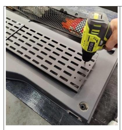
Place the door panel on a flat surface. Place the Molle panel evenly over the indention on the door panel. It is best to have someone else hold it securely in place while you drill 7/32" holes at the INSIDE holes of the Molle panel as shown. Two at each end. You will not use the outside holes.
