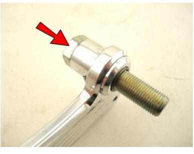
Insert a 1/2-20x2.25 Bolt into the back of the Shifter Pedal.
