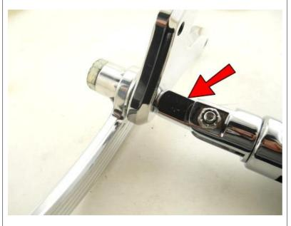
Thread a foot peg onto the 1/2-20x2.25 Bolt and tighten in the desired position.
