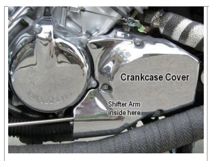
Remove the stock shifter linkage from the ball joint at the shifter arm under the chrome crankcase cover by rotating the linkage clockwise (it is a left hand thread).
