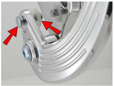
Insert a 5/16x7/8 Clevis Pin into the Brake Pedal, then place a 3/8" Nylon washer onto the Clevis Pin.
