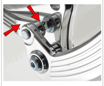
Place the Brake Linkage Extension onto the Clevis Pin, then place another 3/8" Nylon washer onto the Clevis Pin, then a 1/4" Zinc washer and secure with a 5/64x1 Cotter Pin.
