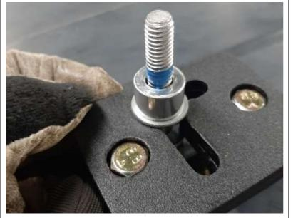
Place another Washer and .5" Spacer onto the Bolt and apply some thread-lock where the nut will go.
