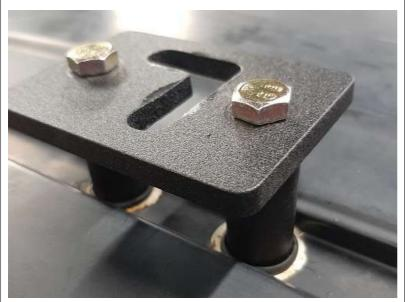
It will be helpful to sit your jack on the roof, close to where you will mount it to decide what the best orientation for the plates will be to hit the holes in the jack best. The plate will work in any orientation; it's just a matter of preference and alignment with your jack.
