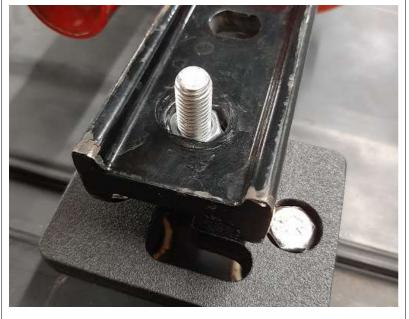
Thread on a 3/8 Nut leaving it loose enough so that you can still slide the Bolt in the slot.
