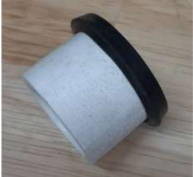
Remove the rubber gasket from the filler tube that came with the Rotopax can.
