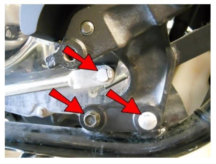
Connect the brake linkage to the ARM11 with the old clevis pin and the supplied 3/64x1 Cotter Pin.
