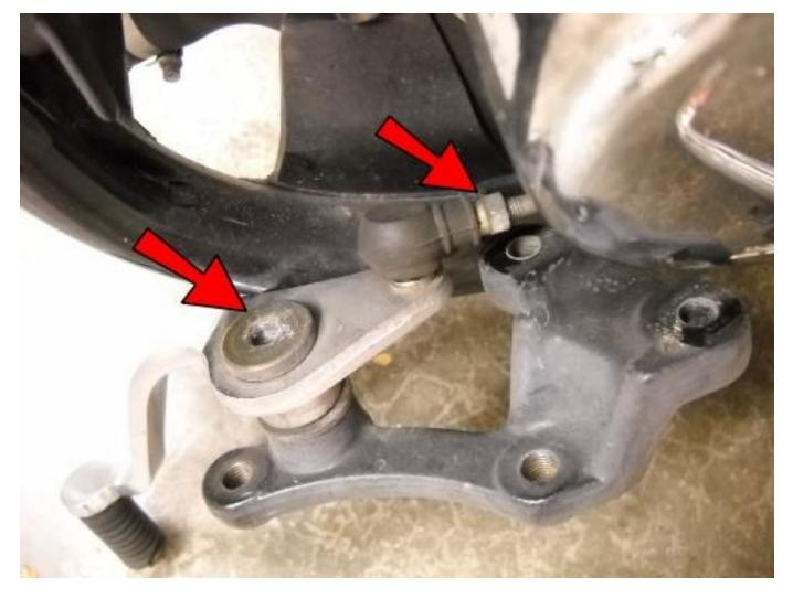
Remove the shoulder bolt that holds the shifter pedal. Loosen the nut on the shifter linkage. Hold the shifter linkage with a pair of pliers and twist the shifter pedal to unthread the ball joint from the linkage. Note: Make sure that you don't unthread the linkage from the rear end while doing this.
