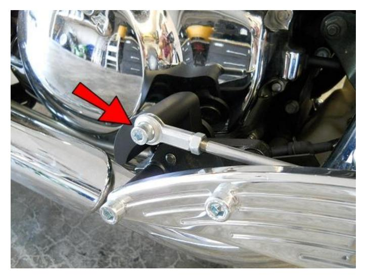
Rotate the linkage around and connect it to the Arm11 with an M8-1.25x25 bolt.
