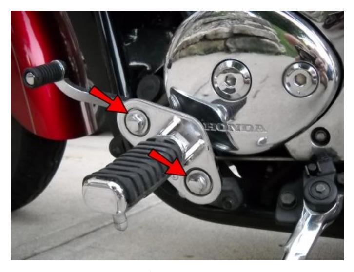
Remove these two bolts on both sides of the bike.
