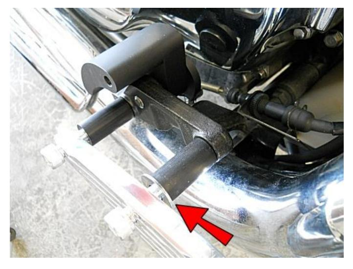
Attach the FC11-R to the old foot peg mount with the supplied M10-1.25x70 bolts, 1.5" Spacers and ONE, 3/8 Washer, on the front, as shown. Note: Depending on which exhaust system you have, you can use more, or NO washers, to adjust for clearance of the brake linkage.
