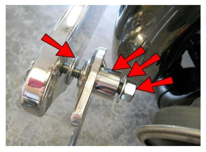
Slide a 5/16 Washer onto the 3/8-16x2.25 bolt that you just installed. Place the Brake pedal assembly on next, then another 5/16 Washer and secure with a 3/8 Nut.
