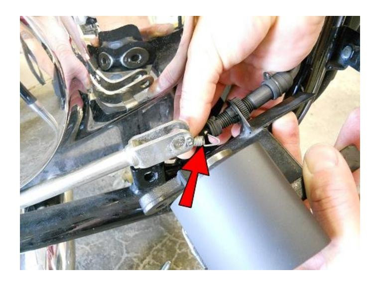
Reconnect the spring to the brake light switch.
