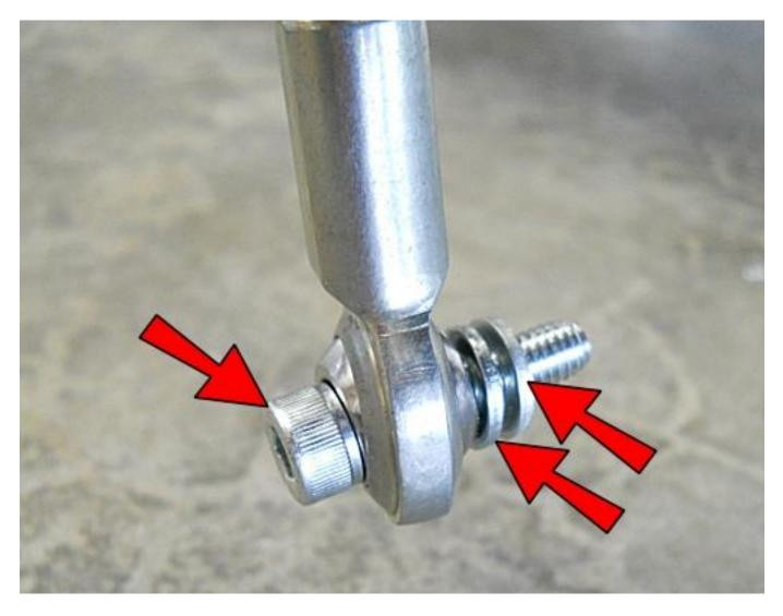
Place another M6-1.0x25 bolt into the other end of the Shifter Linkage, then place TWO M6 Washers onto the bolt as shown.
