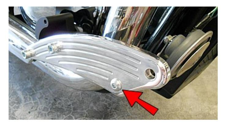
Thread a 3/8-16x2.25 bolt into the bottom hole as shown.
