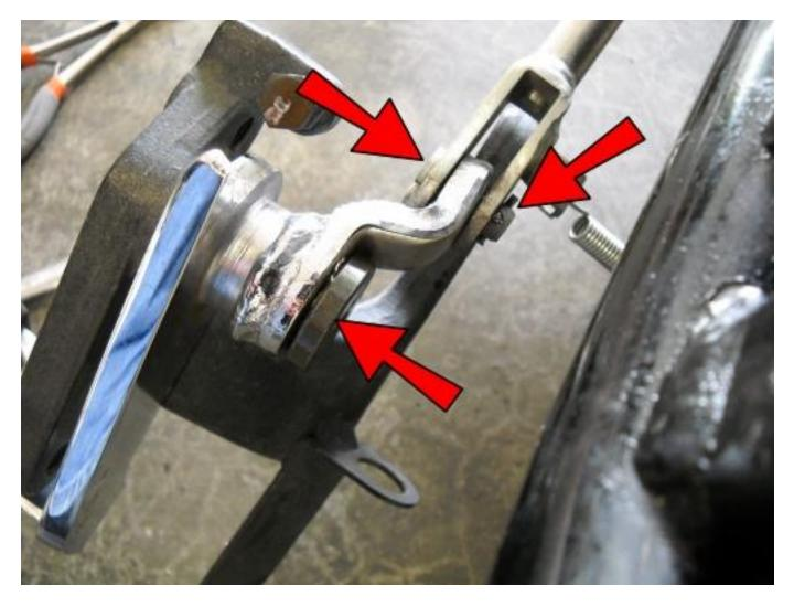
Remove the cotter pin and clevis pin to release the brake linkage, then remove the shoulder bolt that holds the brake pedal.
