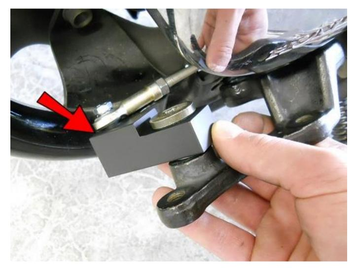
Connect the ARM10 to the shifter linkage as shown.
