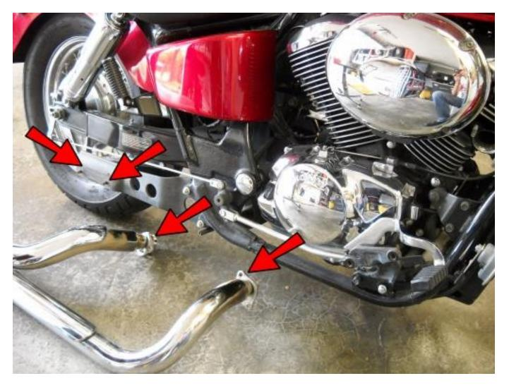
Remove the 4 header nuts and two muffler nuts and remove the exhaust system. Note: You should replace the exhaust gaskets when re-installing the exhaust.
