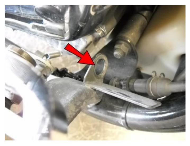
Remove the brake light switch from its mount by gently pulling up.
