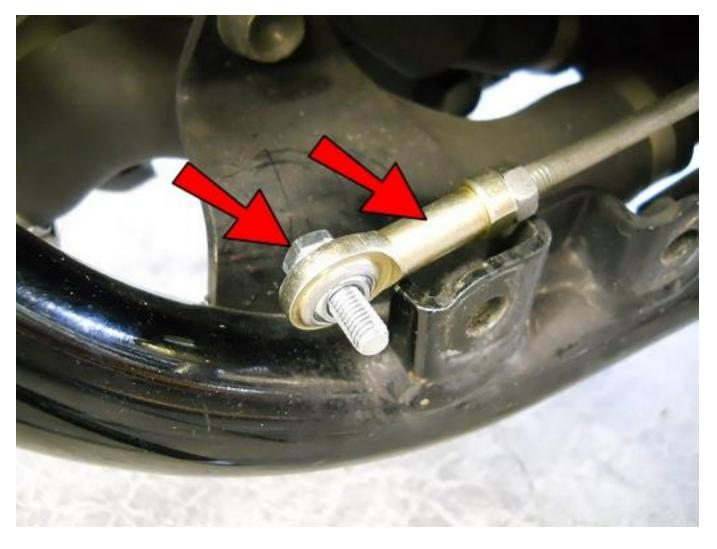
On the shifter side, thread an M6 Spherical Rod End onto the old shifter linkage and place an M6-1.0x20 bolt into the end as shown.
