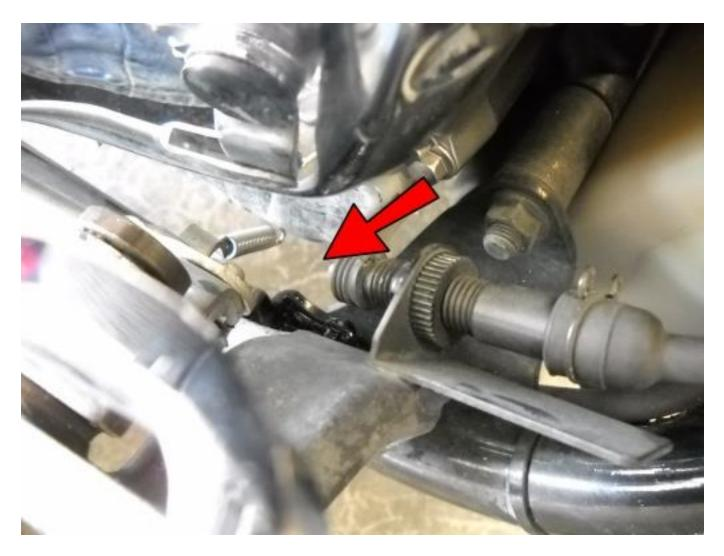
Remove the spring hook from the brake light switch.
