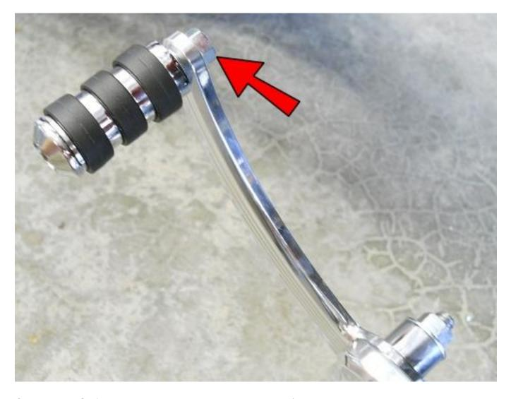
Connect the Shifter Pedal Toe Peg and secure with a 5/16 Nut as shown.
