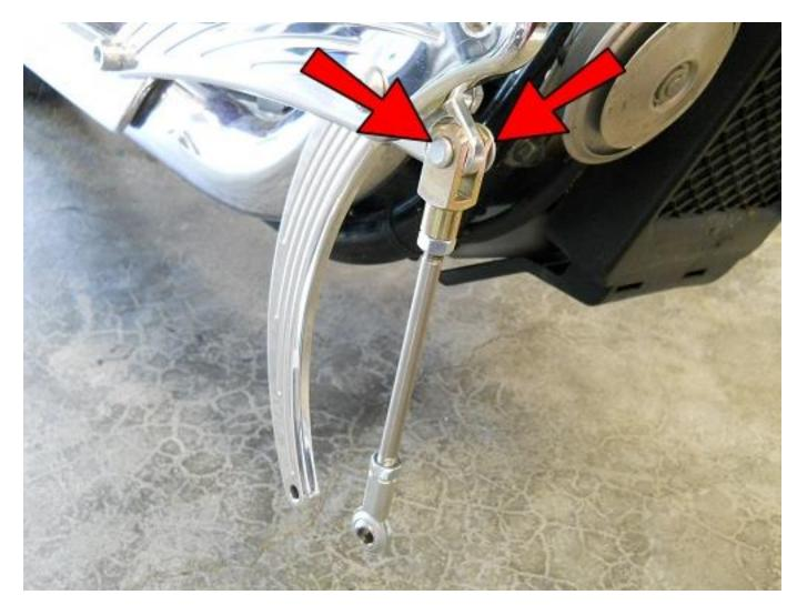
Attach the Brake Linkage to the Brake Pedal with a 5/16 Clevis, 1/4 Washer and 5/64x1 Cotter Pin as shown.
