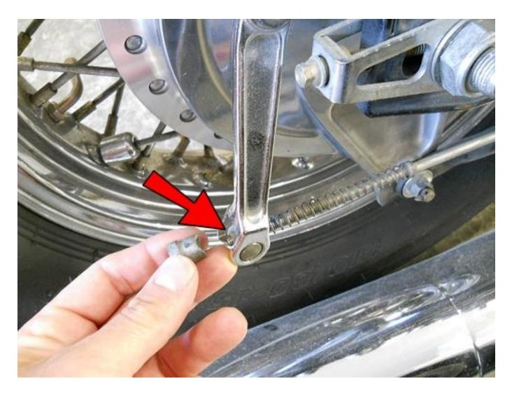
Remove the adjustment nut from the rear brake arm to release the tension on the brake system.
