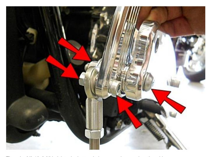
Thread a 3/8-16x2.25 bolt into the bottom hole as was done on the other side.
