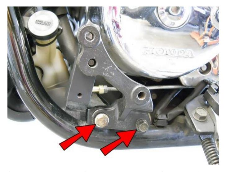
Connect the old mount back to the frame as shown. Then attach the FC11-L to the old foot peg mount with the supplied M10-1.25x70 bolts and 1.5" Spacers, as done on the other side, EXCEPT you will not use a 3/8 Washer on this side.
