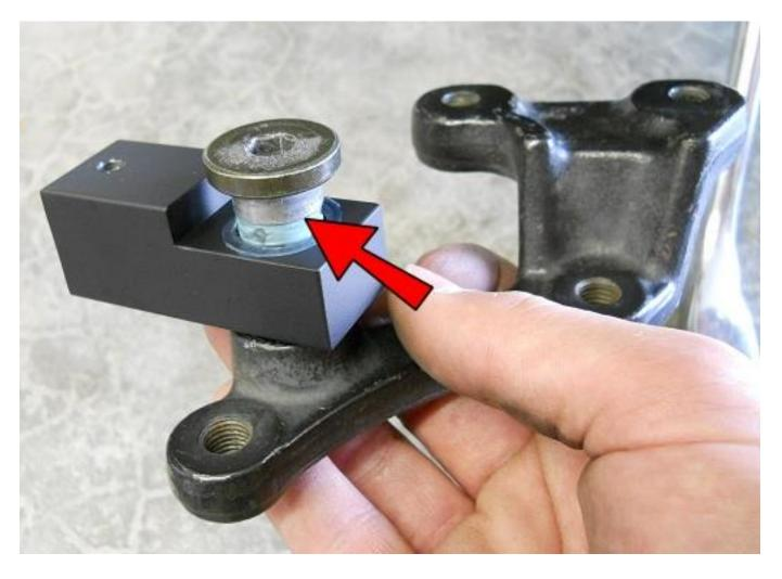
Apply some new grease to the shoulder bolt and use it to connect the ARM10 to the old shifter pedal location.
