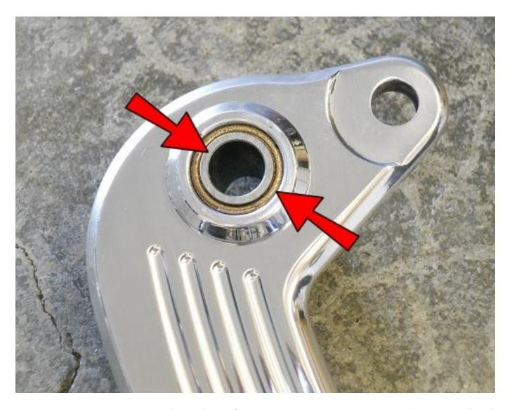
Apply grease to the outside surface of both SLV1's and the inside and outside of both the 5/8x1/2 Bronze Sleeves.
