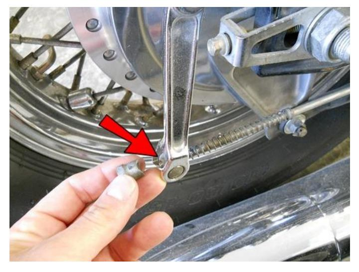
Replace the adjustment nut on the rear brake arm. Push the brake arm all the way forward as you thread the nut on to make it easier to turn. You want very little play in the brake arm, so that when you push the brake pedal, it doesn't have to move far to apply the brakes. However, do not make it SO tight, that the wheel can't turn freely.
