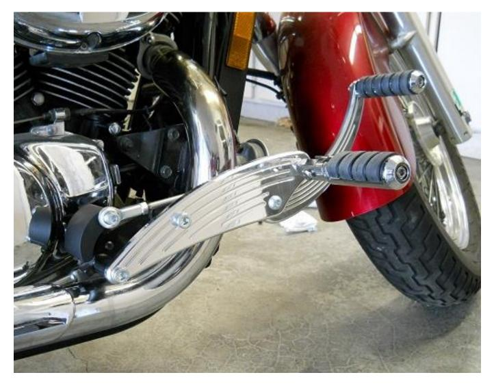
The Brake Pedal height can be raised or lowered by removing one end of the linkage and threading the Linkage Rod into or out of both ends a little. Retighten the 5/16 Nuts when you are finished.
