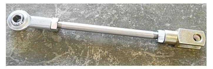
Assemble the Brake Linkage as shown, using a 5/16 Spherical Rod End, a 5/16 Clevis and two 5/16-24 Nuts.
