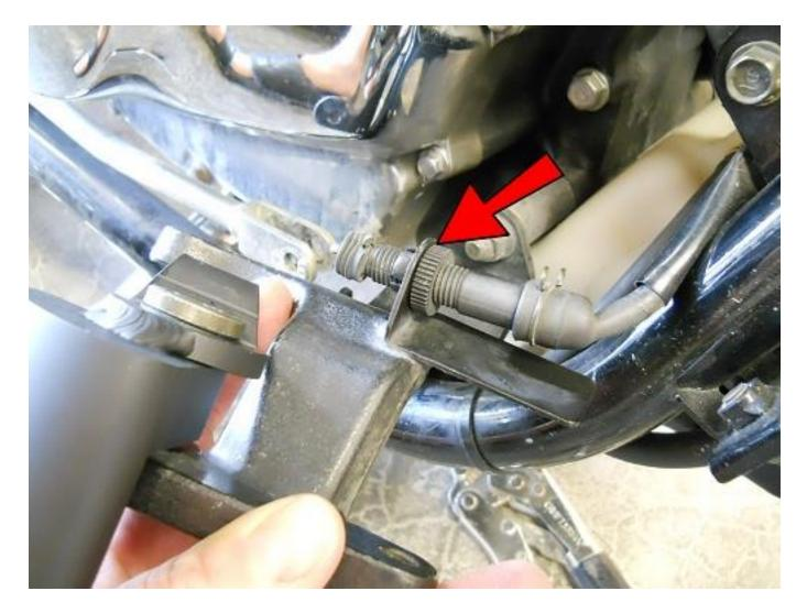
Put the brake light switch back into its mount.
