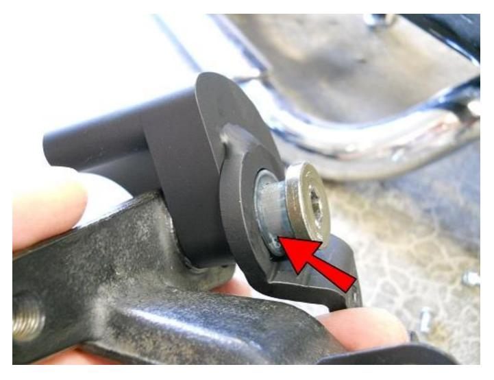
Apply some new grease to the shoulder bolt and use it to connect the ARM11 to the old brake pedal mount.
