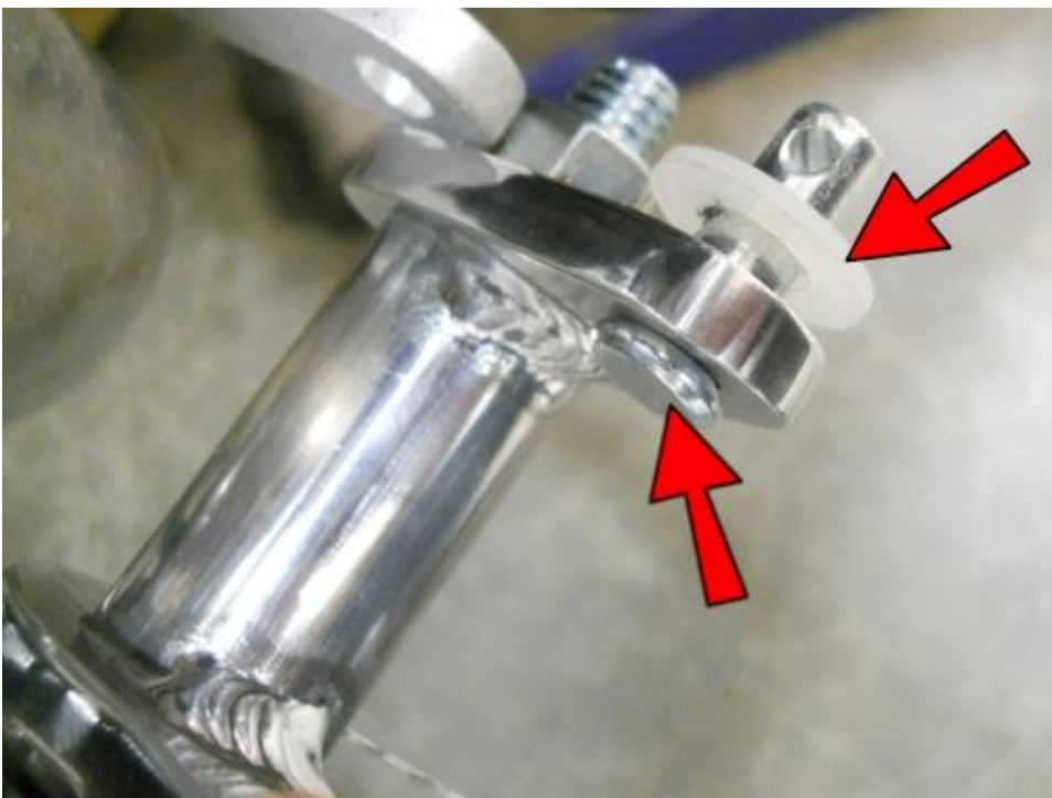
Insert a 5/16x7/8 Clevis Pin into the arm welded onto the Brake Pedal, then place a 3/8" Nylon Washer onto the Clevis Pin.
