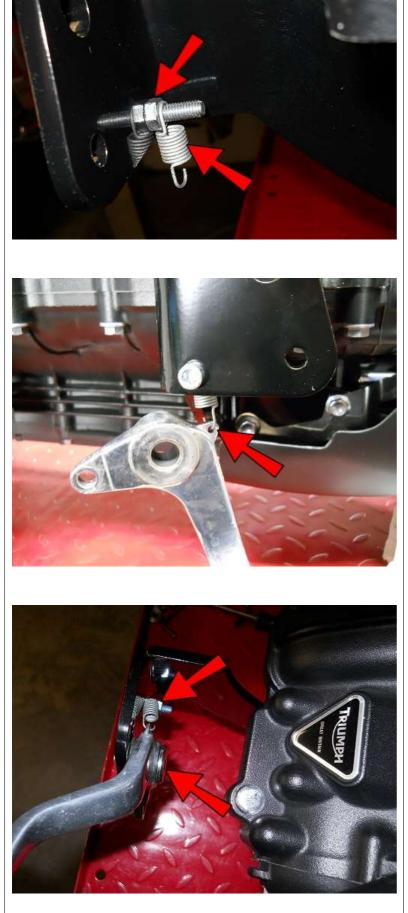
Secure the M6-1.0x25 SHCS with an M6 Nut and hang the brake pedal spring on here.
