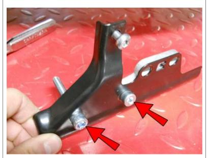
Place the STOF7 onto the inside of the reservoir cover as shown.
