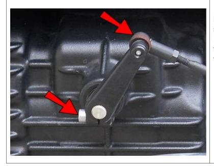
Now remove the spline clamping bolt, then slide the shifter arm off of the spline. Remove the other ball joint end of the linkage from the shifter arm, again using an 8mm wrench under the foam pad.
