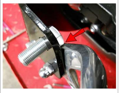
Insert a foot peg bolt so that the flat of the hex head rests against the brake pedal and NOT a point of the hex head, otherwise it will make the pedal sit too low. Note: If you are using any kind of round head, it's fine.
