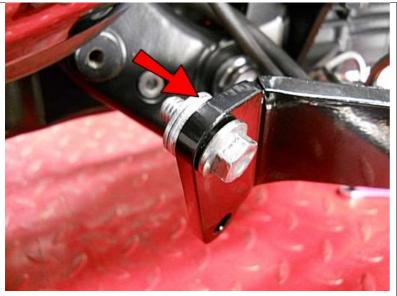
Place one of the original bolts into the top hole of the BSM7, then place three 1/4" Washers onto the back side of it. Note: Do this with this one bolt only.
