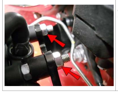
Thread both bolts in ONLY a few turns so that the bracket hangs loose.
