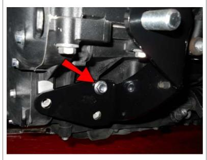
Insert the bolt that will hold your foot peg into the 1/2" hole from the inside as shown.
