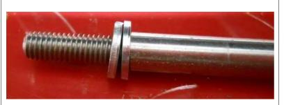
Slide two M6 Washers onto the LEFT hand threaded end of the Brake Linkage.
