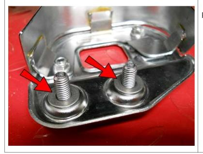
Hold the assembly level and tighten the bolts.
