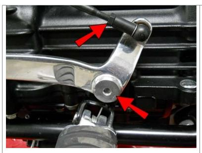
On the shifter side, loosen the locking nuts on BOTH ends of the linkage. Note: the nut on one of the ends (it should be the one on the spline arm, not shown) is a left hand thread. Then remove the shifter pedal bolt.
