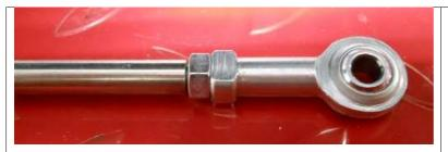
Thread an M6 Nut and a Spherical Rod End onto the RIGHT hand threaded end of the Brake Linkage.
