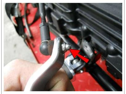
Remove this acorn nut. Note: There is a groove under the little foam pad that holds the stud from turning as you turn the nut. After you loosen the nut a little, you will have to keep the ball joint pressed against the pedal while removing it to hold it in the groove. It may also help to hold the flat of the stud (under the foam pad) with an 8mm wrench while turning the nut.
