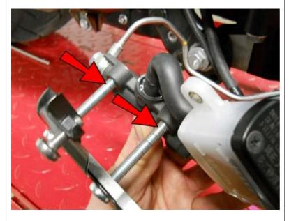
Thread the M8-1.25x60 SHCS all of the way into the master cylinder and tighten.
