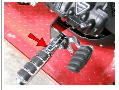
Connect a foot peg, being careful to keep the flat of the hex head as flat against the brake pedal as possible. Each foot peg is different but after adjusting, make sure all connections are tight.
