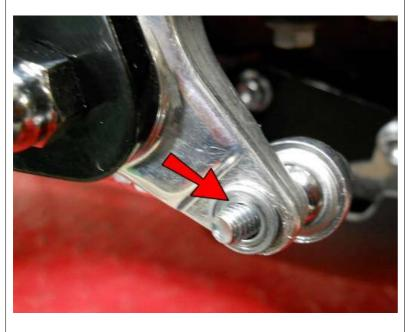
Place it into the brake pedal, then slide another M6 Washer on. Note: make sure the holes line up so that you are not putting tension on the brake, which might cause the brakes to not release fully. If you need to make fine adjustments such as one washer instead of two at the rear of the linkage or adjust the Spherical Rod End, do so. You want it to have no play, but also no pretension on the master cylinder plunger.
