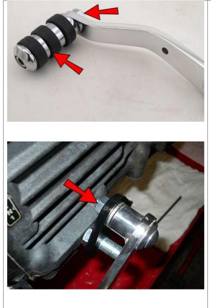
Attach the Shifter Pedal to the FC17-L and secure with a 3/8" Nut.
