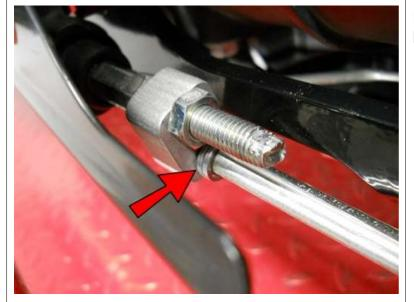
Insert an M6-1.0x25 SHCS into the Spherical Rod End, then slide an M6 Washer on.
