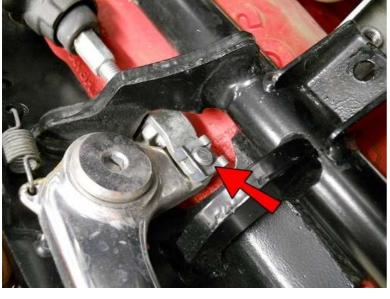
Remove this clip and the clevis pin holding the brake pedal to the master cylinder, then remove the master cylinder from the foot rest assembly.
