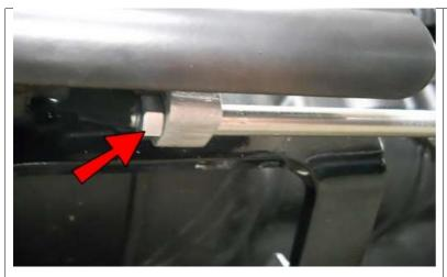
Secure the rear of the linkage with an M6 Left Hand Nut. Note: hold the linkage just in front of the STOF5 with pliers while tightening the nut.
