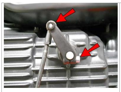
Flip the shifter arm over so the clamping bolt comes in from the rear of the bike and reconnect the ball joint onto the other side, then slide it back onto the spline at about 11:00 o'clock position and secure with the clamping bolt. Note: the end result will basically be a mirror image of how it was originally.
