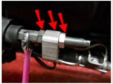
Remove this bolt to remove the brake pedal then remove the spring.
