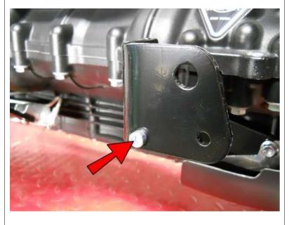
Connect the reservoir cover to the master cylinder cover and secure with M8 Nuts.
