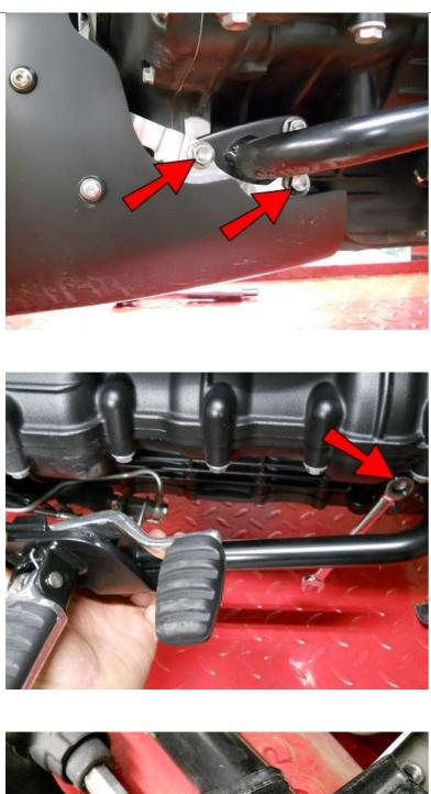
Go to the shifter side and remove only these 2 bolts and remove the chin spoiler if you have one.
