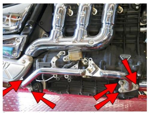
Remove these 5 bolts to remove the stock foot rest mount.
