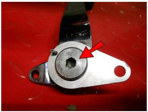
Insert the brake pedal bolt into the brake pedal. Note: Make sure the ARM17 doesn't slip between the hub and bolt head or when you tighten it, the brake pedal won't move freely.
