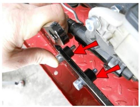
Place 1/2" Spacers on the bolts on the back side.
