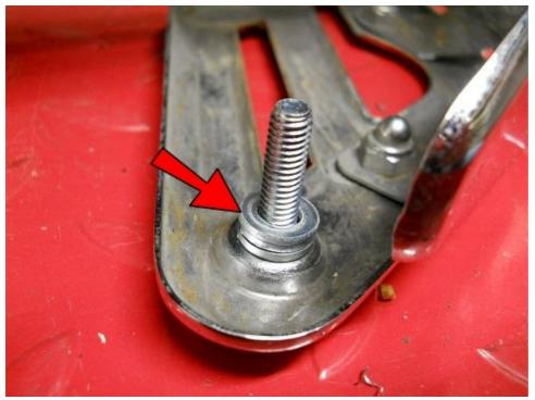
Insert it into the front of the brake reservoir cover, then place three M6 Washers onto it.
