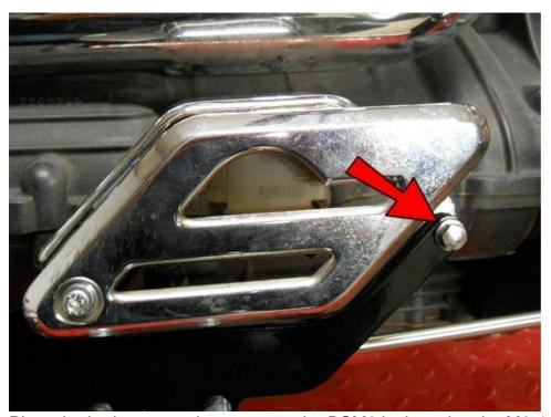
Place the brake reservoir cover onto the BSM8 by inserting the M6-1.0x25 SHCS into the hole and line up the other hole, with the tab behind the BSM8, and secure with the original bolt.
