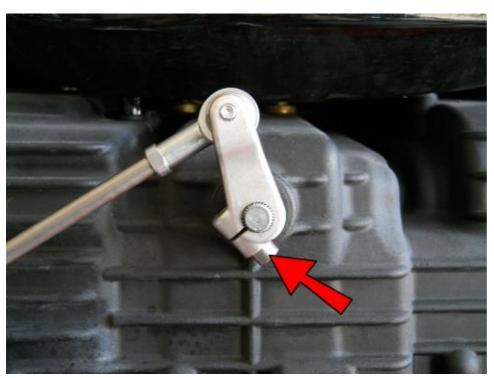
Slide the shifter arm back onto the spline at about the 11:30 clock position and secure with the clamping bolt.
