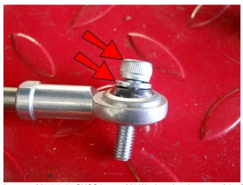
Insert an M6-1.0x25 SHCS into an M6 Washer, then into one of the Rod Ends.
