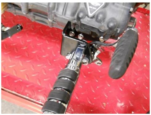
Install a foot peg. Note: The foot peg bolt acts as a stop for the brake pedal.
