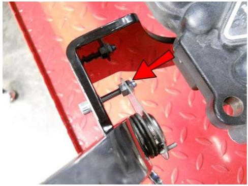
Now secure the ARM17 with another M6 Nut and use 2 wrenches to tighten both nuts against the ARM17.
