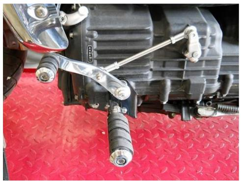
Attach a toe peg and secure with a 5/16" nut, then attach a foot peg.
