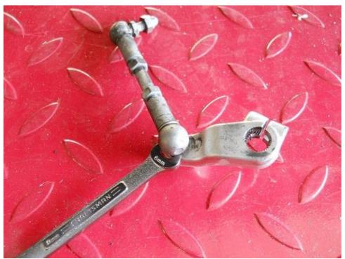
Remove the other ball joint end of the linkage from the shifter arm, again using an 8mm wrench under the foam pad.
