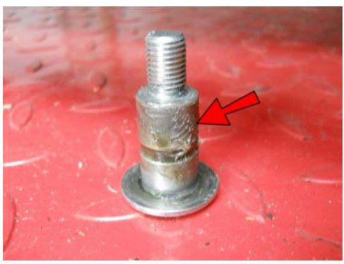
Apply some new grease to the brake pedal bolt.
