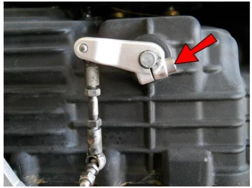
Completely remove the shifter arm clamping bolt, then slide the shifter arm off of the spline.
