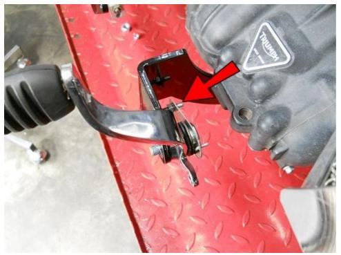
Place the brake pedal assembly onto the FC17-R, making sure the small hole in the ARM17 lines up with the M6-1.0x40 SHCS that you installed earlier.
