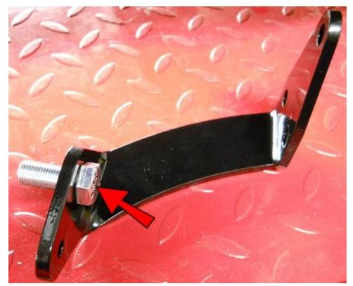
Insert the bolt that will hold your foot peg into the 1/2" hole from the inside as shown.
