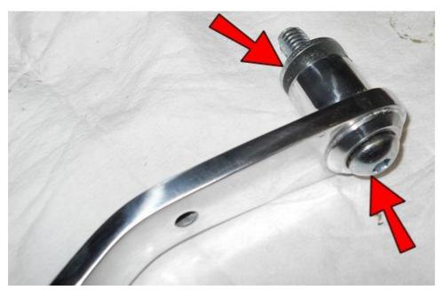
Insert the 3/8 x 2" BHCS into the front and slide a 5/16" Washer onto the back.
