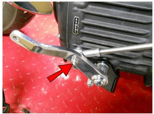
Insert that bolt into the Shifter Pedal and secure with original acorn nut.
