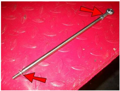
Place an M6 Washer onto one end of the Brake Linkage and thread an M6 Spherical Rod End onto the other end.
