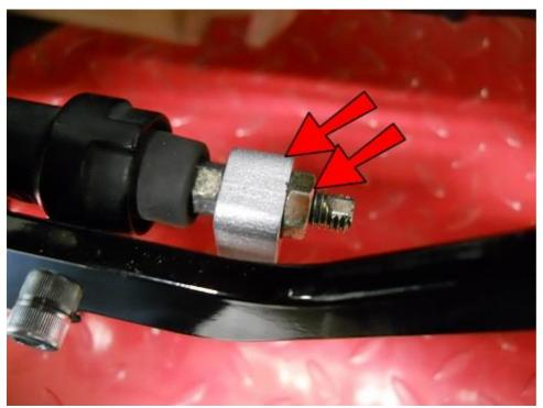
Place a STOF5 onto the master cylinder plunger and secure with the nut you removed previously. Note: Use 2 wrenches; one on the plunger to keep it from twisting and one on the nut, and make sure the STOF5 is very tight. Note: It is ok if the plunger turns while you are tightening it. Just turn it when you are done so the STOF5 hangs straight down.
