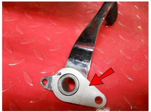
Orient the ARM17 as shown and place it onto the brake pedal hub and insert the spring end into the hole on the ARM17.
