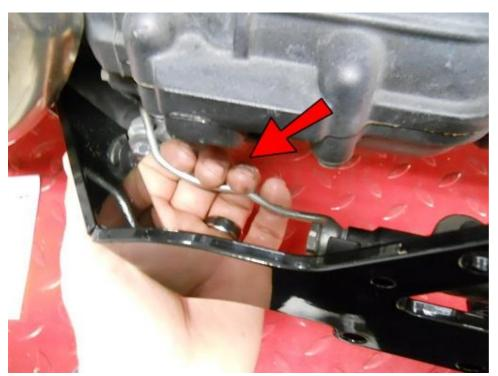
Support the master cylinder in your right hand while you GENTLY and slowly pull the rigid brake line out and back so that it bends to allow the master cylinder holes to line up with the lower holes in the BSM8.
