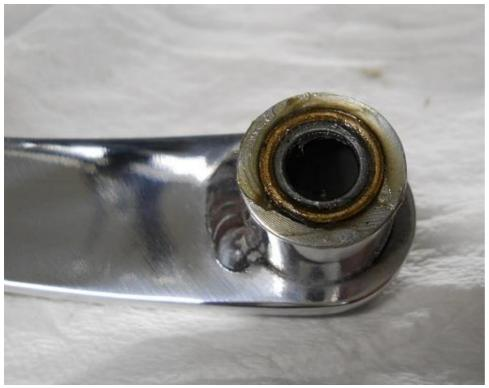
Insert the SLV1 into the 5/8x1/2 Bronze Sleeve, then insert the Bronze Sleeve into the Shifter Pedal.
