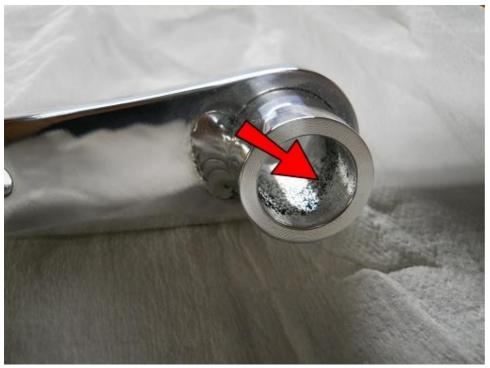
Clean out any polishing compound that may have built up inside the hub of the Shifter Pedal.
