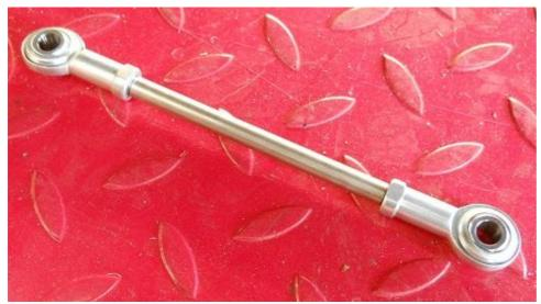
Thread 5/16 Spherical Rod Ends all of the way onto the new Shifter Linkage.
