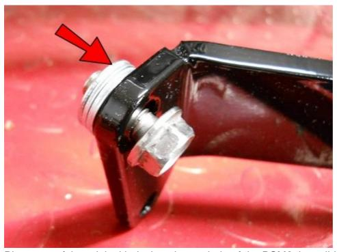
Place one of the original bolts into the top hole of the BSM8 then slide three 1/4" Washers onto the back side of this bolt only.
