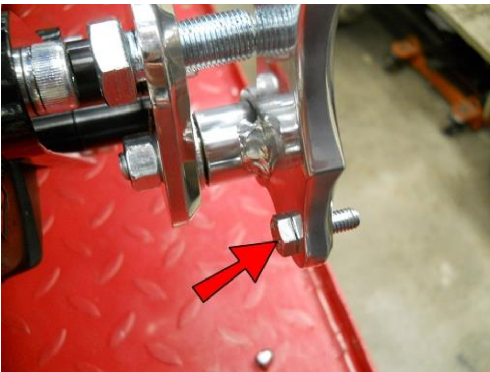
Thread the M6-1.0x18 Bolt into the back side of the Shifter Pedal.
