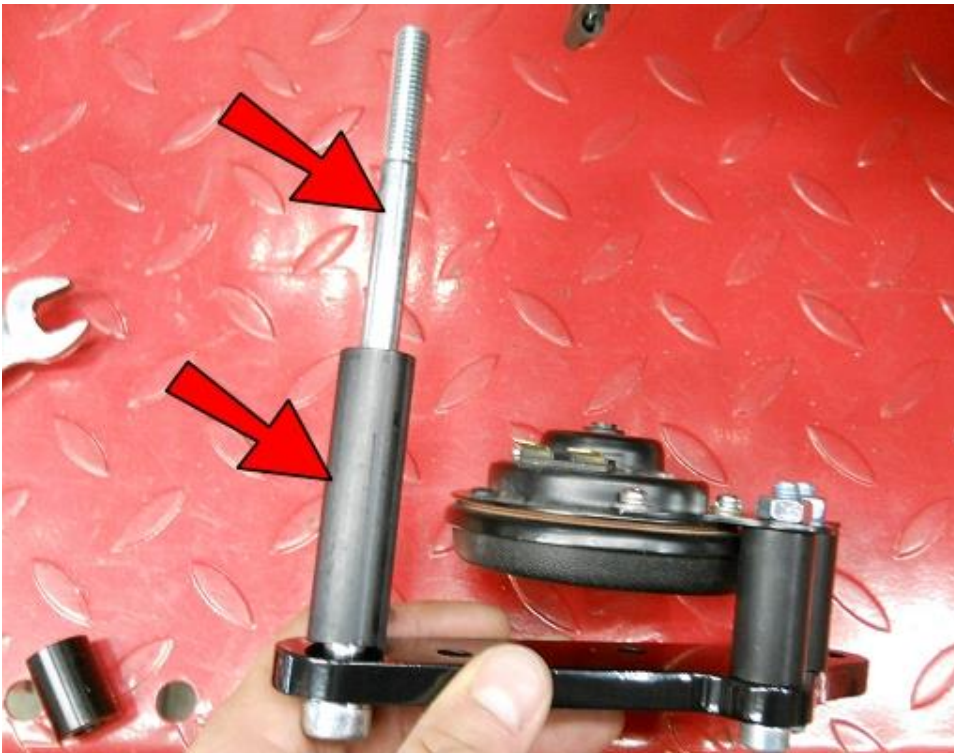
Insert an M10-1.25x170 SHCS and place a 2.8" Spacer on it.
