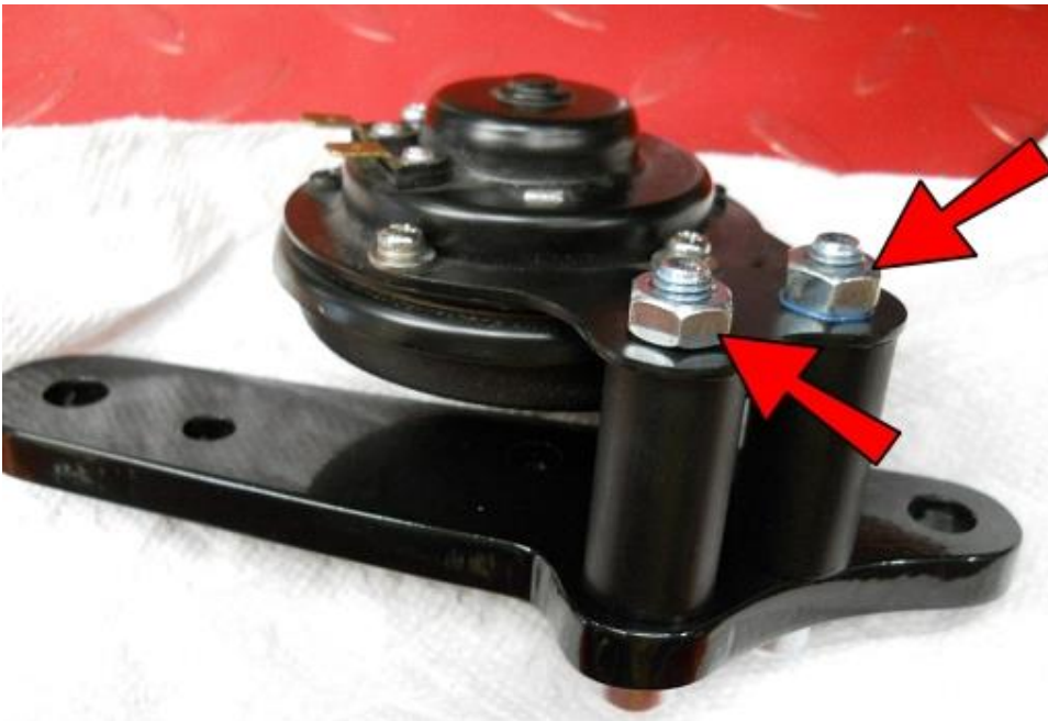
Attach the horn and secure with M8 Nuts.
