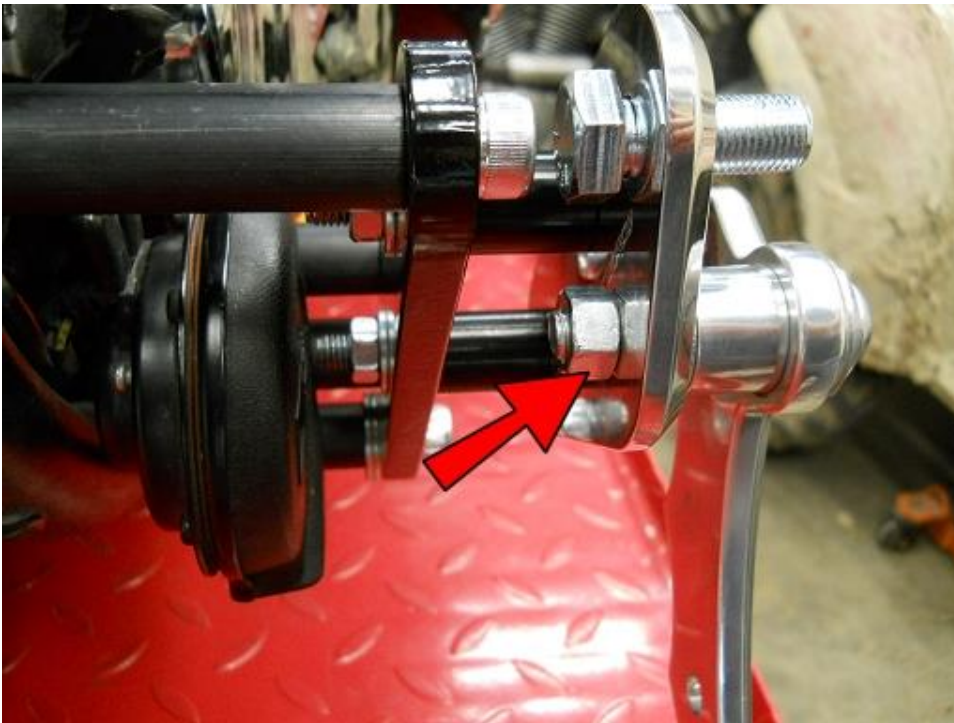
Secure to the Left Control Plate with a 3/8 Nut.
