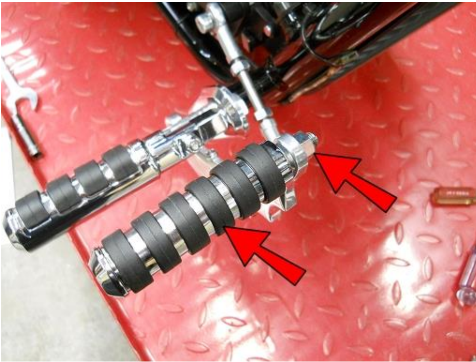
Attach the Brake Toe Peg and Secure with a 5/16 Nut.
