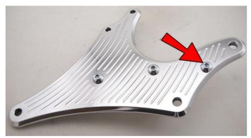
Thread a 3/8-16x2 button head bolt all the way into this hole.
