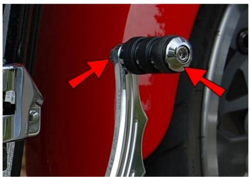
Install a toe peg onto the brake pedal and secure with a 5/16 nut.
