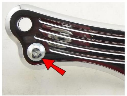
Thread a 3/8-16x2 button head bolt all the way into this hole.
