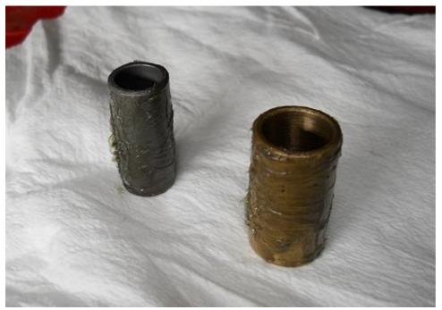
Apply grease to the outside surface of both SLV1's and the inside and outside of both the 5/8x1/2 Bronze Sleeves.
