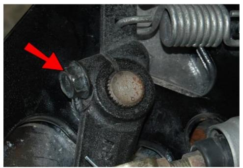
Completely remove this bolt and remove the brake arm from the spline. This will allow the pin holding the master cylinder to fall out and the brake return spring to come off.
