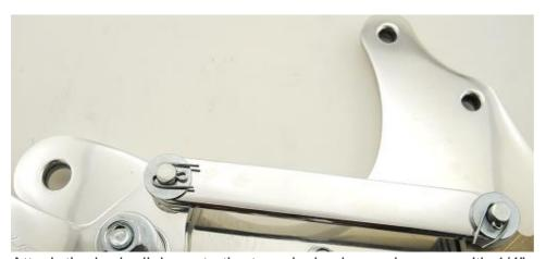
Attach the brake linkage to the two clevis pins and secure with 1/4" washers and cotter pins.
