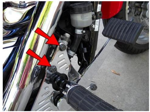
Remove the 2 bolts that hold the master cylinder.
