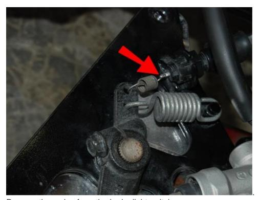
Remove the spring from the brake light switch.
