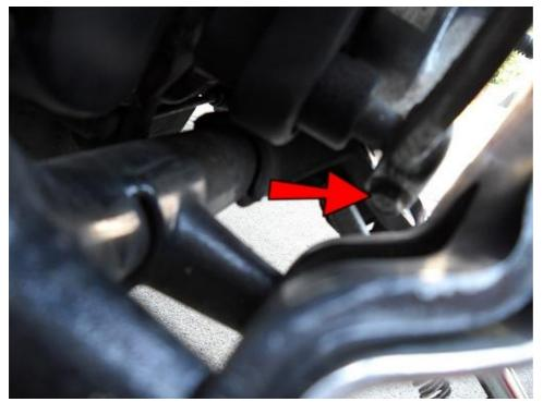
Completely remove the shifter pedal spline bolt and remove the shifter pedal from the spline.
