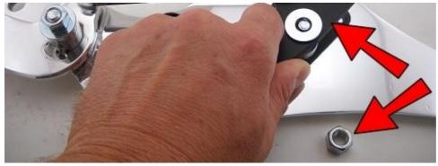
Now work the ARM4 back onto the spacer and secure with the 3/8 nut.
