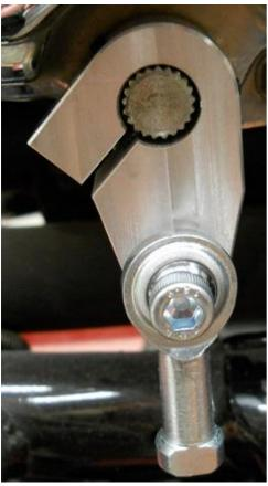
With the screwdriver still in place, slide the ARM3 onto the shifter spline and orient the ARM3 pointing down and just slightly to the right as shown. Line up the bolt hole on the top of the ARM3 with the groove in the spline and remove the flat screwdriver.
