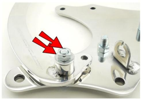
Place the Brake Pedal assembly onto the 3/8-16x2 Button head bolt and secure with a 5/16 zinc washer and a 3/8 nut.
