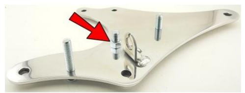
Thread a 3/8-16 nut on here and tighten.
