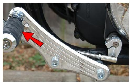
Install a foot peg onto the FC5-L.
