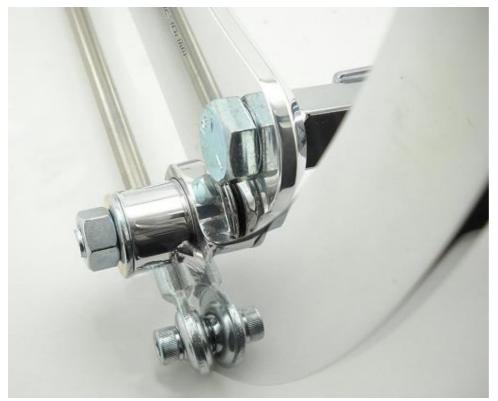
Connect the shifter linkage to the back of the Shifter pedal using an M6-1.0x25 socket head bolt and secure with an M6-1.0 acorn nut.
