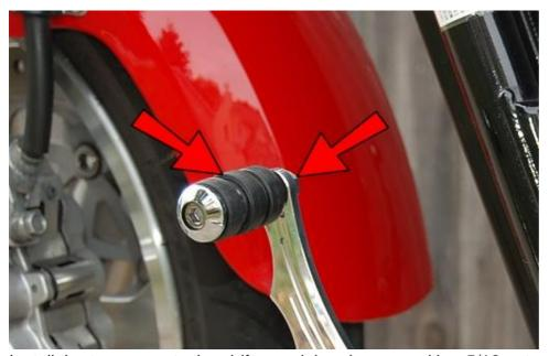
Install the toe peg onto the shifter pedal and secure with a 5/16 nut.
