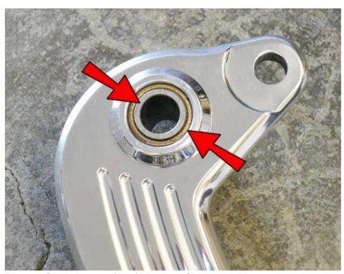
Place a SLV1 into a 5/8x1/2 Bronze Sleeve and insert them into the Brake and Shifter Pedals.
