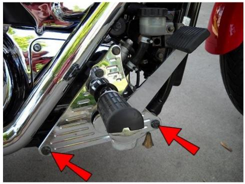
Remove the 2 bolts at the bottom. On the frame tube, behind the rear bolt location there is a hose stay holding the brake hose to the frame tube. Bend that away and remove the hose from it.
