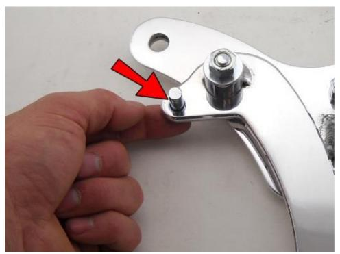
Rotate the brake pedal as far as it will go counter clockwise and insert a clevis pin into the front side of the brake pedal.
