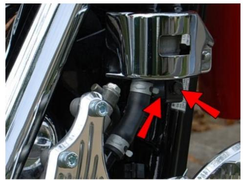
Reattach the brake reservoir to the frame using a .75" spacer and an M6-1.0x30 bolt then reattach the brake reservoir cover. Note: We have had a couple of oddball bikes (literally less than 1%) that required an adapter bracket to relocate the reservoir. Please contact us if you think you may need this bracket.
