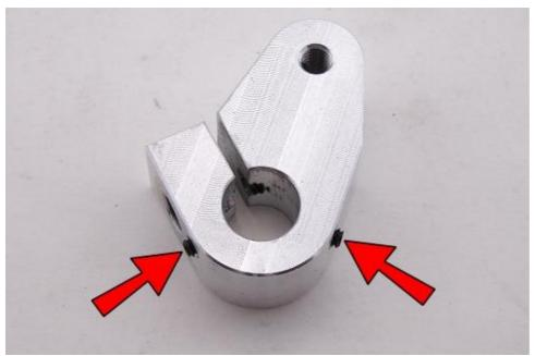
Start the two #6-32 set screws in the small threaded holes of the ARM3 being careful not to let them protrude through yet.
