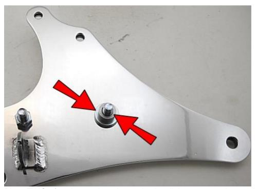
Place TWO 5/16 zinc washers here. Apply a little grease to the outside of the small aluminum spacer and place on top of the washers.
