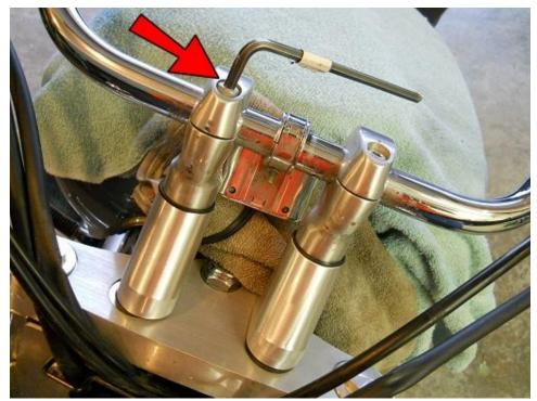
Loosen the riser top clamp so that you can slide the riser over to line it up with the hole, attach it with the other 1/2-20x2.25" bolt and tighten both bolts.
