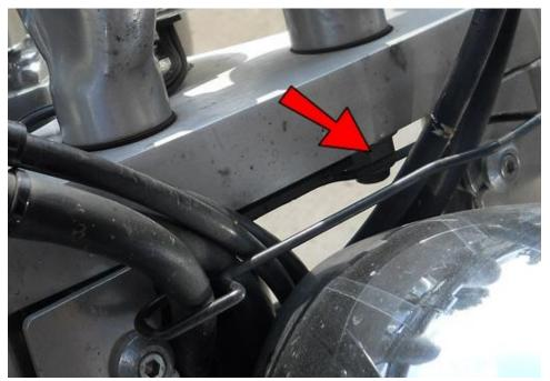
Remove the nut holding the risers to the triple tree and remove the risers.
