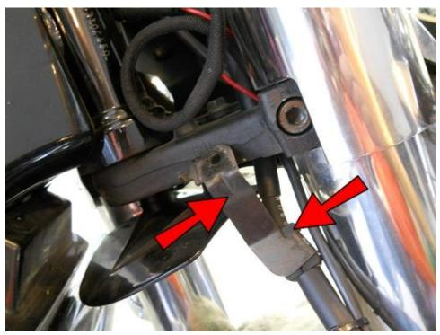
Remove the bolt holding this retaining clip, then remove the retaining clip and rubber grommet from the hose.
