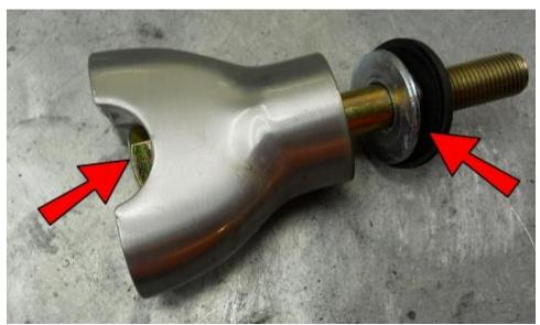
Remove the stock bolt from both risers and place a 1/2-20x4" bolt into them, then replace the zinc washer, then the rubber washer.
