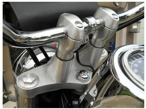
Loosen the other riser top clamp, adjust the bars to the desired position, and tighten.
