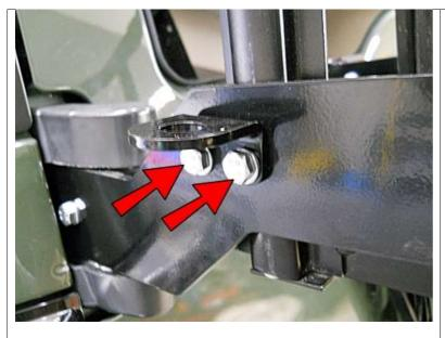
If installing the Optional CB Antenna Mount, use the supplied M6-1.0x20 Hex Head Cap Screws in this corner INSTEAD of the M6-1.0x18.
