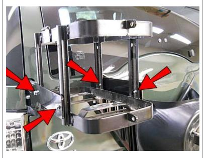
Put the holder in place and insert the 4 remaining M6 Screws with Washers into the corner holes.
