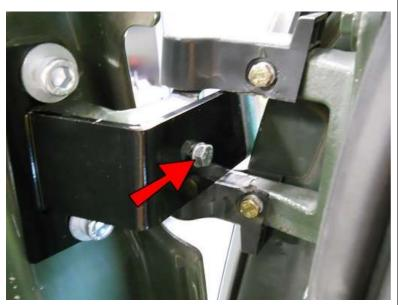
Insert it into this hole and make sure it goes all the way into the hole in the hinge. You may need to jiggle the Bracket to get the holes to line up.
