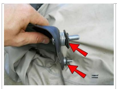
On the other two Screws on the right side of the spare tire carrier, place THREE 3/8" Zinc Washers and one of the rubber washers removed earlier onto each one.
