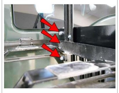
Now go back to these 3 Screws on the Right Side Bracket and one at a time, remove the nuts, apply thread lock and tighten.
