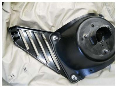
Place the JM1 Main Bracket onto the two Screws on the left side of the carrier.
