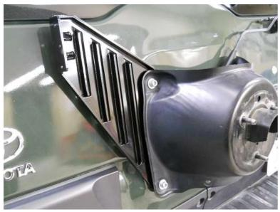
Being careful not to let the carrier or the Main Bracket touch the paint, thread all 4 Screws into the carrier mounting holes on the door. Thread them most of the way, but leave them loose enough that you can move the Main Bracket up and down.
