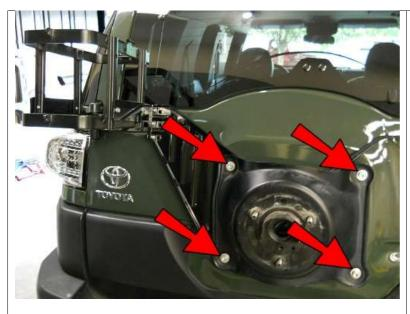
Finally, tighten these Screws completely. Note: Since they are on a rubber washer, they will not feel completely tight, so just get them very snug.
