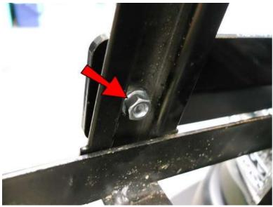
Now secure all corners with M6 Washers and Nuts. Don't forget to use thread lock!
