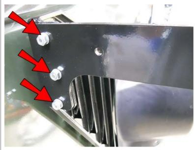
Place the JM1 Right Side Bracket onto the Screws and thread three M6 Washers and Nuts onto them and only finger tighten at this time.
