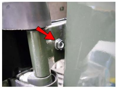
Apply some thread lock to the M6-1.0x30 Screw previously inserted and secure with an M6 Washer and Nut.
