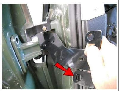
Insert the JM1 Left Side Bracket through the hinge as shown. If you tilt it at the correct angle it will go easily, don't force it, just try another angle if it isn't going
