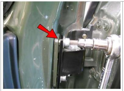
Line up the holes of the Left Side Bracket to the hinge and use the M10 Screws with Washers and Sleeves to connect the Bracket. Make sure the Alignment Sleeves go into the alignment holes on the Left Side Bracket AND the hinge. Do NOT tighten yet.
