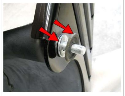
Place a 3/8" Zinc Washer and one of the rubber washers removed earlier onto the back side of those two M10 Screws. Later models had a thin stick on plastic washer instead of the nice thick rubber ones. If your washers are not reusable you can get the stick on ones from Toyota, Part #51998-35020 or you can wrap some electrical tape around the Zinc Washer to protect the paint.
