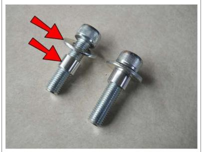
Place a 3/8" Zinc Washer and an SPC036 Alignment Sleeve onto 2 of the M10-1.25x40 Socket Head Cap Screws as shown.
