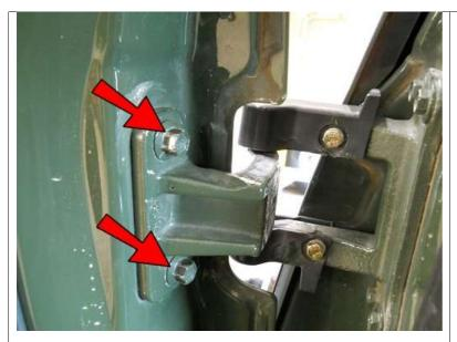
Remove the hinge bolts. (Again, make sure the door is firmly supported, it is heavy!)
