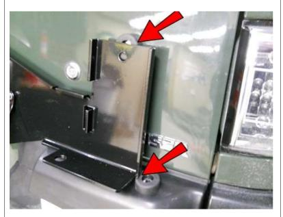
Remove the towel that you had wrapped around this end and rest the right side bent edge on a bumper and if you haven't already installed a bumper at the top using the No Drill Method, then just slide one in for spacing as shown, then go ahead and tighten all four M10 Screws holding the tire carrier on.
