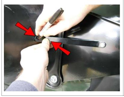
Hold the Brace level and push it against the carrier with one hand as you mark the hole with the other.
