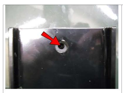
Using the Bumper hole as a guide and the same 1/4" drill bit used earlier, drill just a quick center mark on the door.
