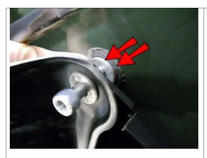
Place the JM2 onto the two Screws on the right side of the carrier. Place a 3/8" Washer and one of the rubber washers removed earlier onto the back side and hand tighten only.
