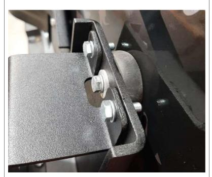
Insert the other 2 bolts with washers into the 2 holes on the top of the optional bracket then into the JM2. (Your bracket may differ slightly).
