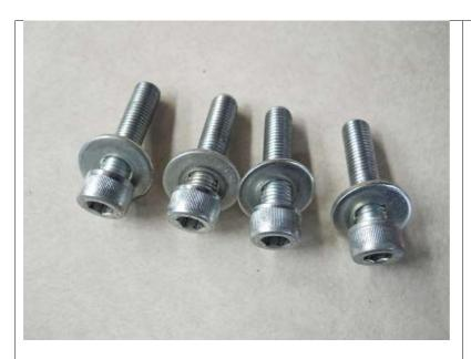
Place a 3/8" Washer on each of the four M8-1.25x40 Socket Head Cap Screws.
