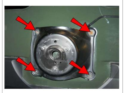
Remove the two bolts and the two nuts holding the spare tire carrier to your door. When you remove the carrier, there will be 4 rubber washers on the bolts or stuck to the paint surface. If they are loose, carefully peel them off. If they are the newer, thinner style and are adhered pretty well, just leave them there. Either way, you will re-use them. If yours are torn up or you just want a replacement, they don't make the thick ones anymore so look into Toyota part # 51998-35020
