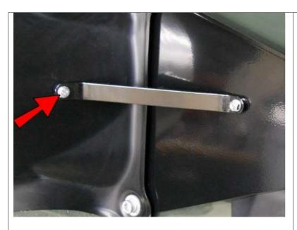
Place the Bolt into the Brace and into the JM2.
