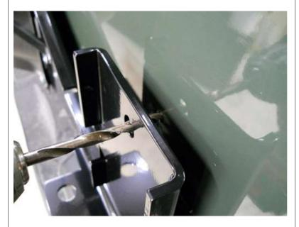
Remove the Bumper for now and drill the hole completely through the door. Then put a dab of paint on the exposed metal to protect it.
