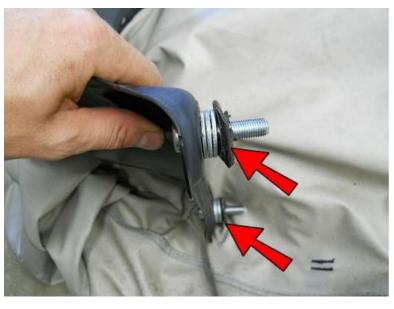
On the LEFT side of the spare tire carrier, place THREE 3/8" Washers and one of the rubber washers removed earlier onto each one. (Note: If you also have our JM1 or JM3, only use 1 washer here.)
