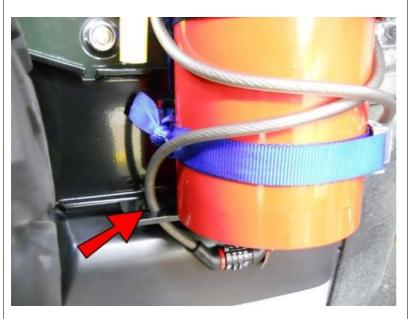
This hole is for locking your cylinder to your JM2 Mount. You can use a bike combo lock cable as shown or any other cable or chain secured with a padlock in that hole. If you are mounting a fire extinguisher, remember to remove the lock prior to hitting the trail so it is readily available!
