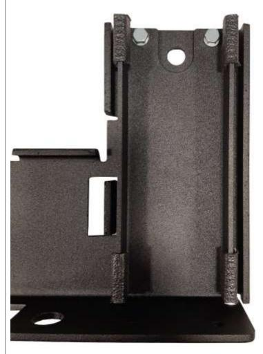
For any cylinder smaller than 8" diameter, attach an optional Small Dia. Adaptor Kit as shown, using the bolts, washers and nuts and place the 4 Edge Trim pieces on the adaptor as shown.
