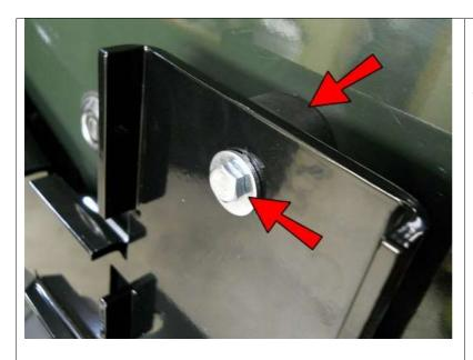
Put the bumper back in place, with the FLAT edge toward the door. Center it on the hole, making sure the top edge is flush with the top edge of the JM2 and insert the Bolt.
