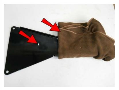
Insert the Bolt and Washer into the back side of the JM2 as shown, then flip it over and wrap a towel around the end of the JM2. This will protect from scratching your paint or the plastic door handle cover while installing.
