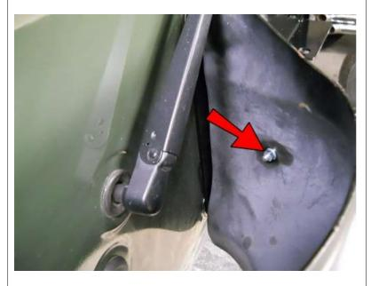
Secure with an M6 Washer and M6 Nut. Don't forget that Loctite mentioned at the beginning!
