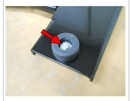
Place the Bolt and Washer into the recessed side of the 5/8" Rubber Bumper and into the hole from the back of the JM2 as shown.
