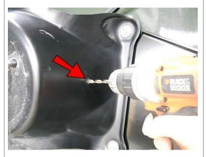
Drill a 1/4" hole on your mark. Then put a dab of paint on the exposed metal to protect it.
