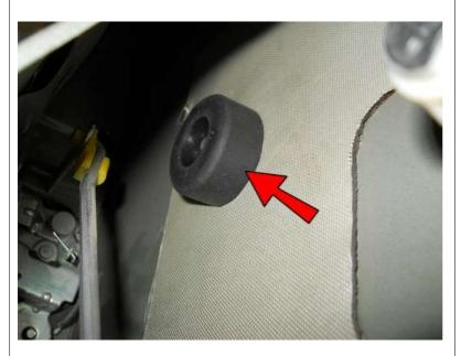
Place another Bumper on the bolt on the inside of the door, again with the FLAT edge toward the door. Secure with an M6 Washer and M6 Nut. It will not get completely tight because you are just squishing the rubber. Get it snug so that you can see the rubber on the outside of the door slightly compressing. Then add a second M6 Nut. Loctite is very important on this one in particular.
