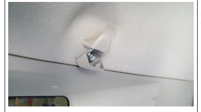
Snap open the cargo area hanger hook to access the M6 screw and remove it from both sides of the vehicle.
