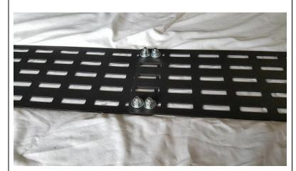
Flip the Panels <u>over</u> and lay the other ends, one on top of the other, and insert the remaining four 1/4-20x1/2 Carriage Bolts from the <u>BOTTOM</u>. Place Washers on top and <u>ONLY START</u> the 1/4-20 Lock Nuts. DO NOT TIGHTEN the Lock Nuts.
