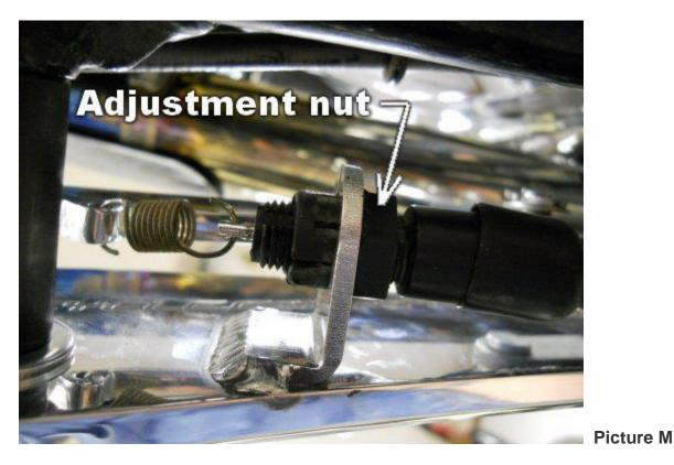
Hold the brake light switch in one hand to keep it from turning, while using a wrench to turn the nut. If the spring tension is too tight, your brake light will be on all of the time. If it is too lose, it will not come on when the brake is applied.
