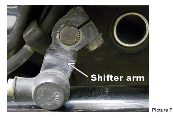
Hold the Shifter Pedal in the position you want, and slide the shifter arm back onto the spline and secure with the bolt previously removed from the shifter arm. After testing, the position of the pedal can be adjusted by rotating the shifter arm or by threading the Shifter Linkage in or out. After adjustment is finished, make sure to tighten the nuts on both ends of the Shifter Linkage to secure it.
