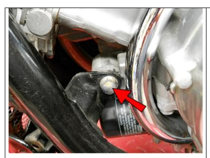
Remove this motor mount bolt and nut.
