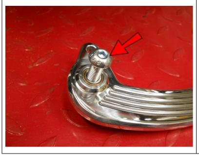
Insert a 3/8-16x2" Button Head Bolt into the Brake Pedal.
