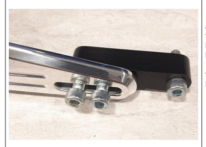
Insert two M8-1.25 x 30mm bolts into the slot at the rear of the Shifter side plate and thread them half way into the two threaded holes of the V65 Extension with the other hole toward the rear. Insert the other M8-1.25 x 30mm bolt into the V65 Extension and thread into the front stock foot peg mount hole.
