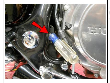
Press the brake pedal down, then place a large screwdriver behind the middle brake arm to keep it forward as shown.
