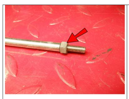
Thread that nut all the way onto the new Shifter Linkage on the Left Hand Threaded end.
