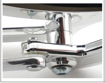
Orient the Brake linkage with the small spring hole toward the rear and attach it to the brake pedal by inserting the clevis pin first into the linkage, then into a Nylon washer, then into the brake pedal, then into a 5/16 zinc washer and secure with a Cotter pin.
