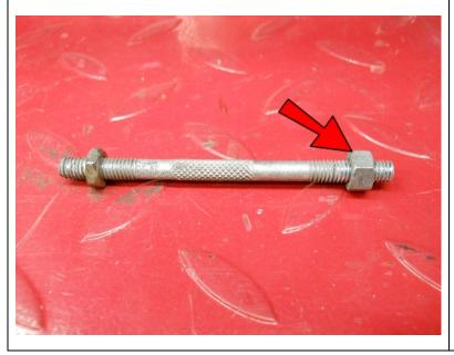
Remove the M6 Left Hand Nut from the linkage.
