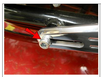
Go back and completely tighten the M8 bolt.
