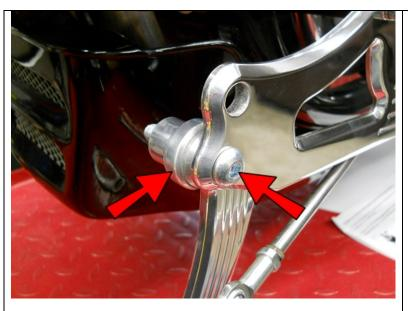
Insert a 3/8-16x2" Button Head Bolt here, then into the Shifter Pedal assembly.
