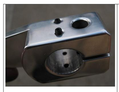
Start the 4 Set screws into the Brake arm and assure they do not protrude through the other side into the large hole.
