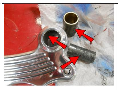
Apply grease to the inside of the hub of both Pedals, the outside surface of the SLV1's and the inside and outside of the 5/8x1/2 Bronze Sleeves.
