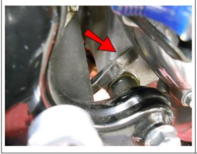
For the next steps below, you may find it helpful to place a large screwdriver behind the frame and use the edge of the motor as a pry point, to put pressure on the back side of the middle brake arm to keep it from sliding in as you install our Brake Arm.
