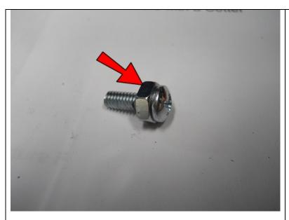
Thread a #8-32 Nut onto a #8-32x1/2" Screw.
