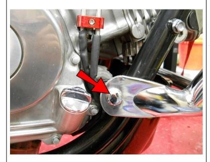
Remove this motor mount bolt and IF you have a case guard as shown here remove it entirely. You will not be able to use it with forward controls.
