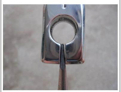
Hold the brake arm firmly and insert a large flat head screw driver into the end and carefully tap the handle of the screwdriver on a hard surface to spread the spline opening apart. The goal here is to spread the hole just far enough apart to easily slide the brake arm onto the brake spline. Note: This can be easy OR the most frustrating part of the install if the hole is not spread apart enough, (but only just enough, not too much).
