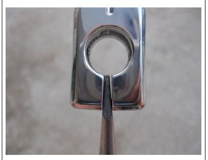
Hold the brake arm firmly and insert a large flat head screw driver or better yet, a small chisel, into the end of the Brake Arm and carefully tap the handle on a hard surface to spread the spline opening apart. The goal here is to spread the hole just far enough apart to easily slide the Brake Arm onto the brake spline. Note: This can be easy OR the most frustrating part of the install if the hole is not spread apart enough, (but only just enough, not too much).
