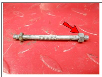
Remove the M6 Left Hand Nut from the linkage.
