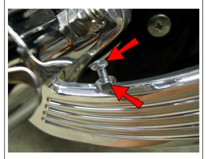
If desired, adjust the angle of the Brake Pedal by unscrewing the #8 Screw, then tighten the Nut against the Brake Pedal to secure.
