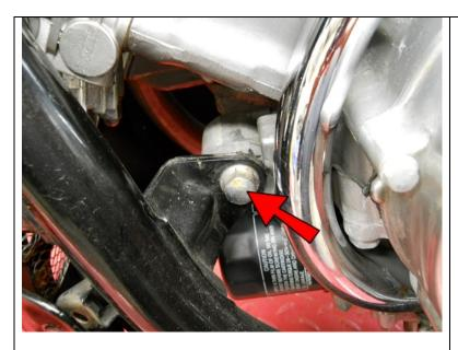
Remove this motor mount bolt and nut.
