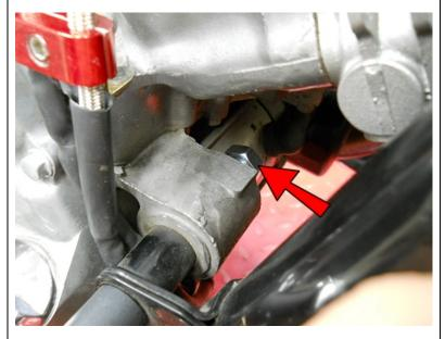
Now secure the M10 Bolt with an M10 Nut on the back side of the motor mount.
