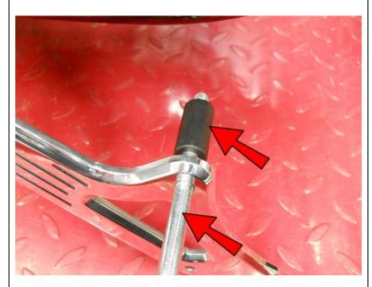
Insert an M10-1.5 x 130mm Bolt into the top hole of the Plate then place a 1.5" Spacer on the bolt.
