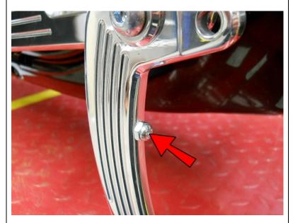
Thread the Screw into the hole in the Brake Pedal.
