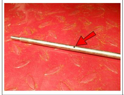
Orient the Brake Linkage with this small hole toward the rear of the bike.
