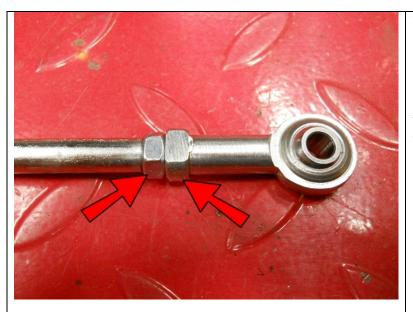
Thread an M6 Nut and M6 Spherical Rod End all of the way onto one end of the linkage and the M6 Left Hand Nut and M6 Left Hand Spherical Rod end all of the way onto the other end. The end of the Linkage with the small hole should be the Left Hand threaded end but if not, it does not make a difference.
