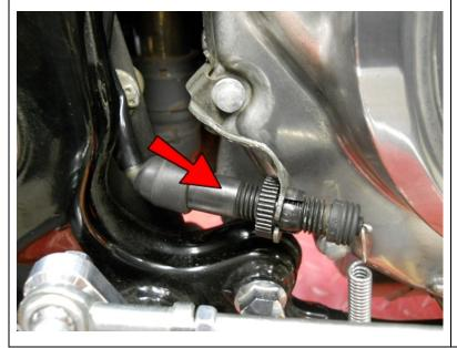
Insert the brake light switch back into the mount.
