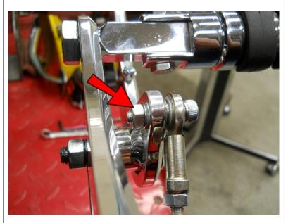
Secure with an M6 Zinc Washer and M6 Nut.
