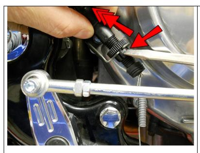
Remove the brake light switch by pressing in the plastic tabs on the adjustment wheel and gently pulling it out of the mount.
