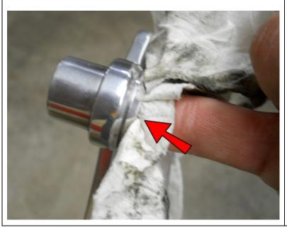
The inside of the Brake and Shifter Pedals will likely have some polishing compound residue. Use a cloth or paper towel and make sure the inside is ABSOLUTELY clean. This can affect how well your Pedals will rotate.
