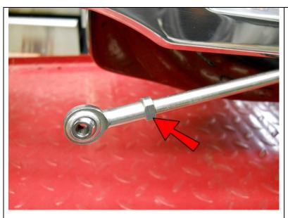
Thread an M6 Spherical Rod End all of the way onto the other end.
