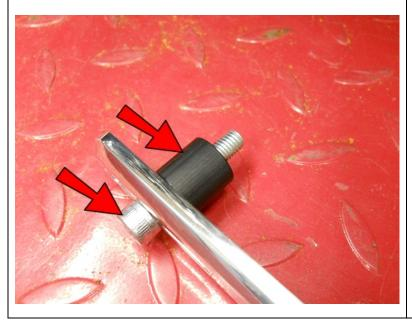
Insert an M8-1.25 x 45mm bolt into the rear slot of the Brake Side Plate then place a 1" Spacer on the bolt.
