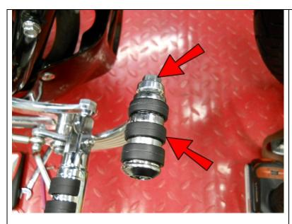
Install a Toe Peg and Secure with a 5/16" Nut.
