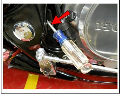
Push the Brake Pedal forward and remove the screwdriver. The Brake Pedal should rest against tightly against the foot peg clevis.
