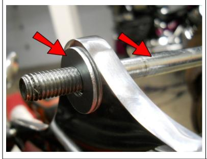
Insert an M10-1.5 x 170mm Bolt into the top hole of the Shifter Side Plate then place a 3/8" Zinc Washer onto the bolt.
