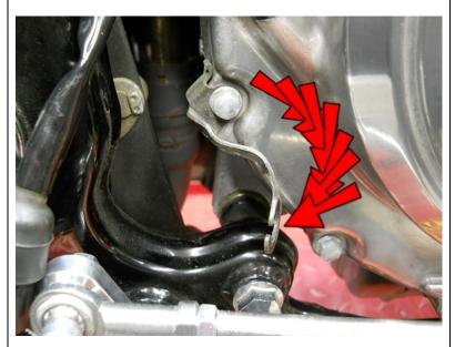
Use pliers to bend the brake light switch mount as shown. Bend slowly and carefully as not to break this mount, they are no longer available from Honda. You can purchase replacement mounts from RefinedCycle.com however.
