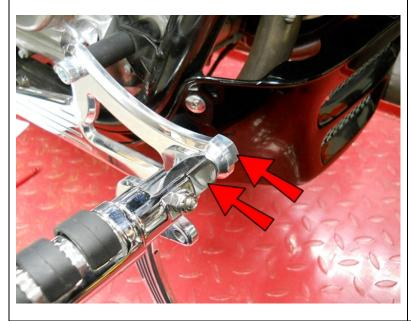
Attach a Foot Peg and Secure with included bolt.
