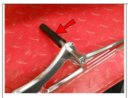
Slide a 4.1" Spacer onto the bolt.
