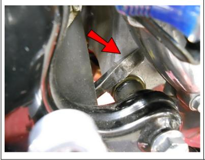
For the next step below, you may find it helpful to place a large screwdriver behind the frame and use the edge of the motor as a pry point, to put pressure on the back side of the middle brake arm to keep it from sliding in as you install our Brake Arm.
