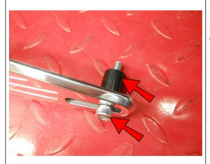
Insert an M8-1.25 x 45mm Bolt into the Shifter Side Plate then place a .75" Spacer onto the bolt.
