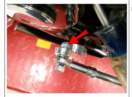
Secure with an M6 Zinc Washer and M6 Nut.
