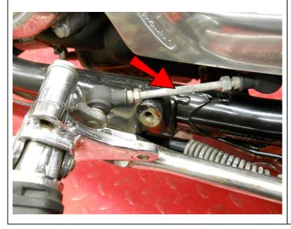
Rotate the linkage rod to unscrew from both ends.
