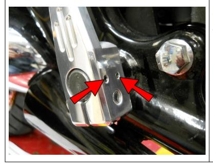
Tighten all 4 set screws in the Brake Arm AFTER tightening the bolt in the above step.
