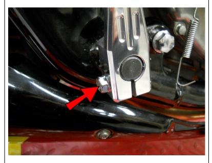
Thread the bolt that came out of the stock brake pedal into the Brake Arm and tighten well. If the threads don't catch, tap the head of the bolt lightly to get it started.
