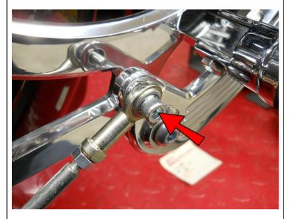
Place the Linkage on the Brake Pedal and insert an M6-1.0x25 Bolt.
