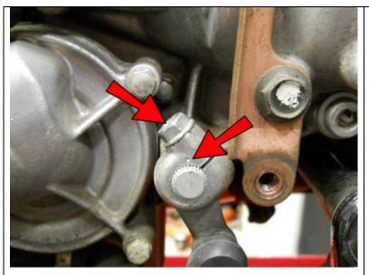
Rotate the shifter arm 1 notch counterclockwise then replace it onto the spline. Place the bolt back into the top and tighten. Replace cover.
