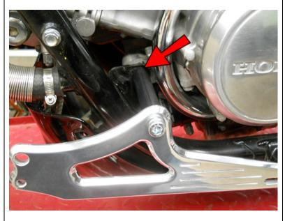
Insert into the motor mount hole and secure with an m10 Nut, then go back and tighten the rear M8 Bolt.
