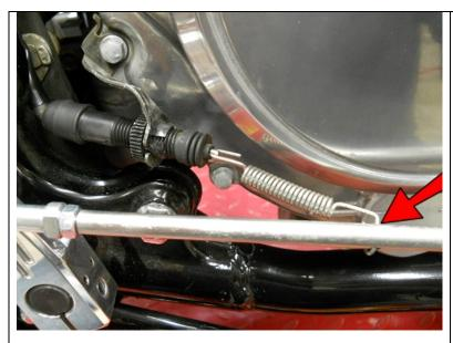
You will also need to bend the spring hook to allow it to fit into the hole on the brake linkage.
