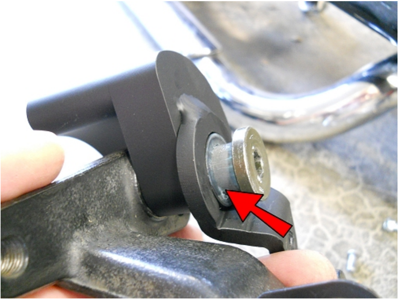
Apply some new grease to the shoulder bolt and use it to connect the ARM11 to the old brake pedal mount.
