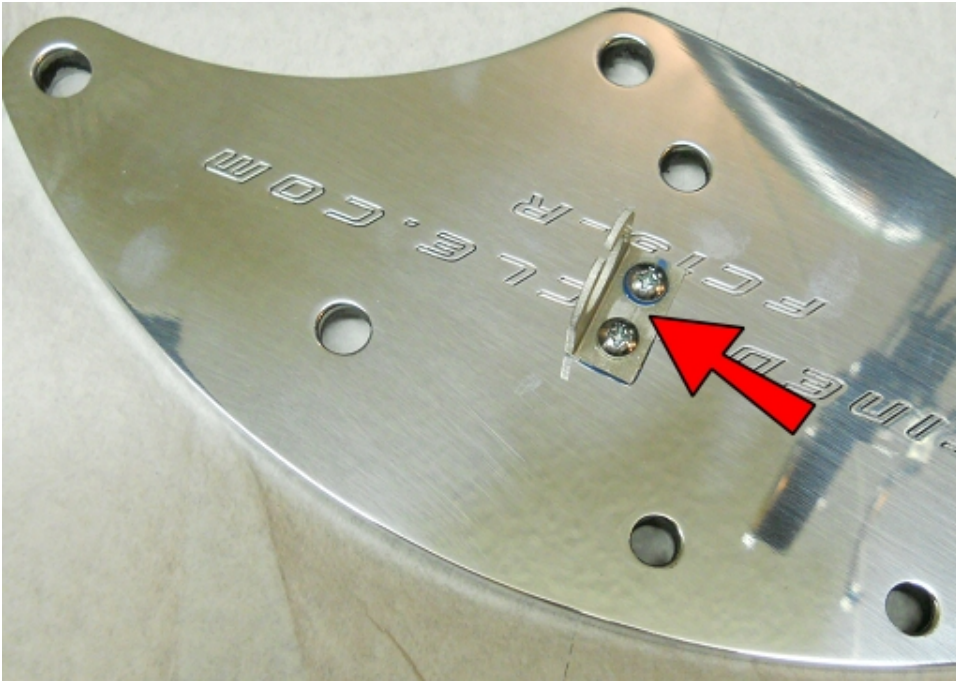
Attach BSM3 to the FC13-R with two #8-32x5/16 Screws.
