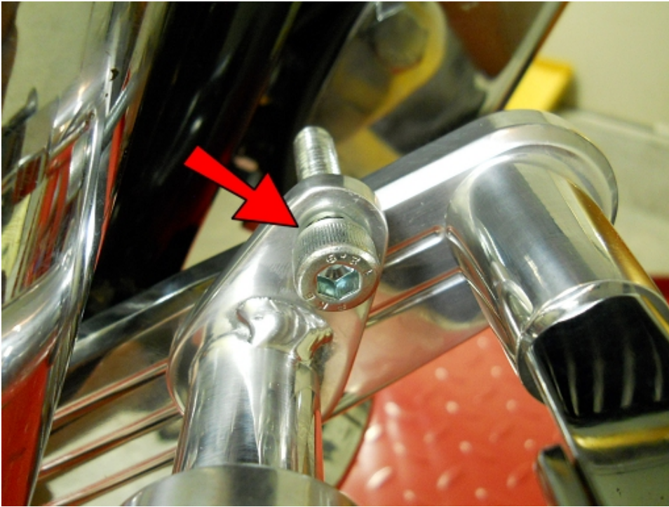
Insert an M8-1.25x40 Socket Head Bolt into the Brake Pedal.
