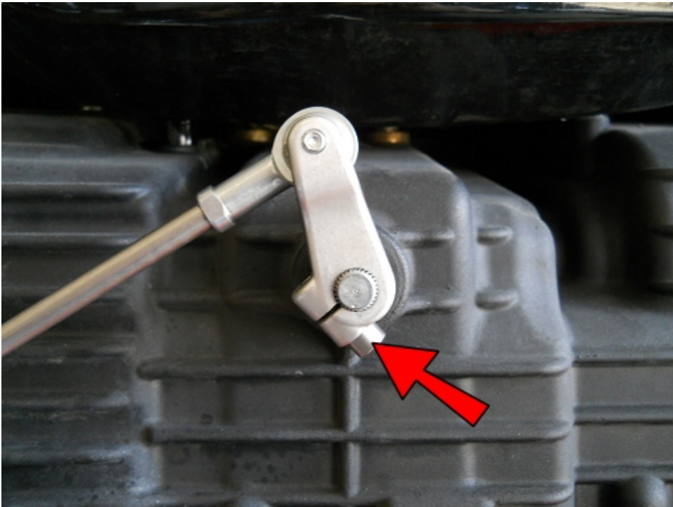
Slide the shifter arm back onto the spline at about the 11:30 clock position and secure with the clamping bolt.
