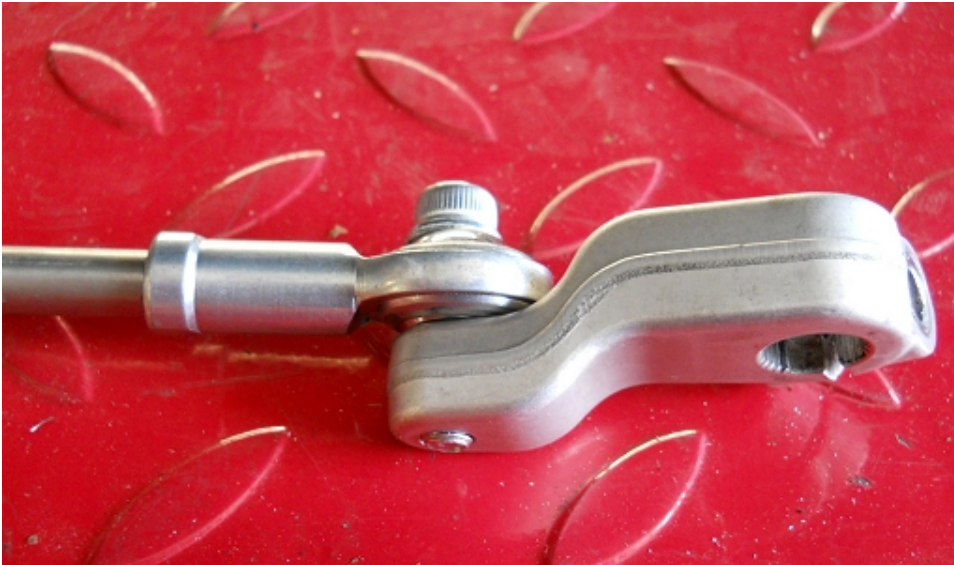
Now connect that end to the shifter arm as shown.
