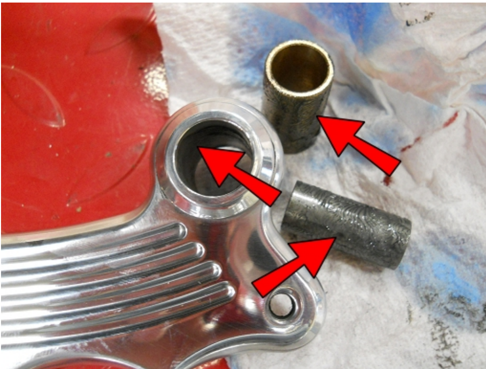
Apply grease to both SLV1's and 1/2" Bronze Sleeves and the Shifter and Brake Pedals.
