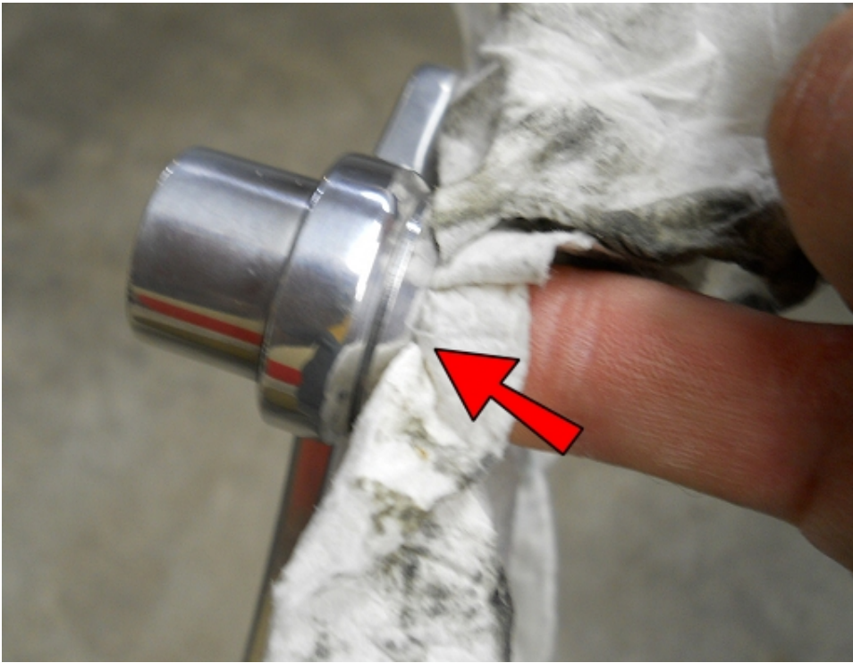
Use a paper towel or cloth to clean the inside of the hubs of the Shifter and Brake Pedals.
