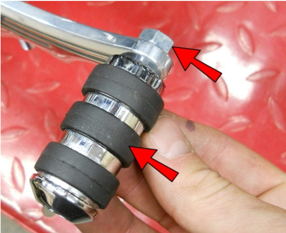
Connect a Toe Peg and Secure with a 5/16 Nut.
