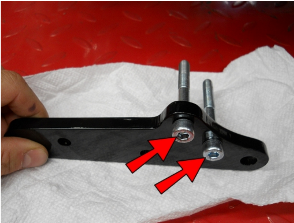
Insert two M8-1.25x60 SHCS's into the STOF9.
