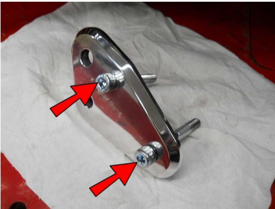
Insert M8-1.25x60 SHCS into these holes of the Left Side Control Plate.
