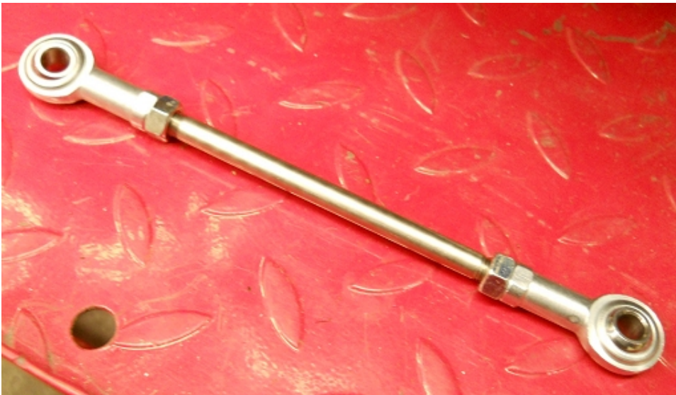
Thread 5/16" Nuts and 5/16" Spherical Rod Ends most of the way onto both ends of the supplied Shifter Linkage.
