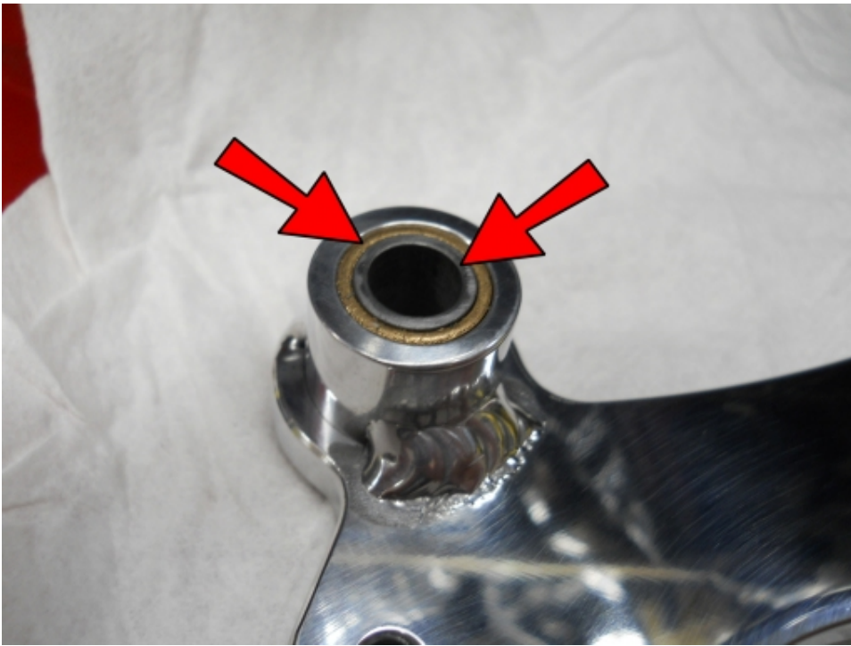
Insert the last set of greased Sleeves into the Shifter Pedal. Remember to make sure the inside of the shifter hub is clean!
