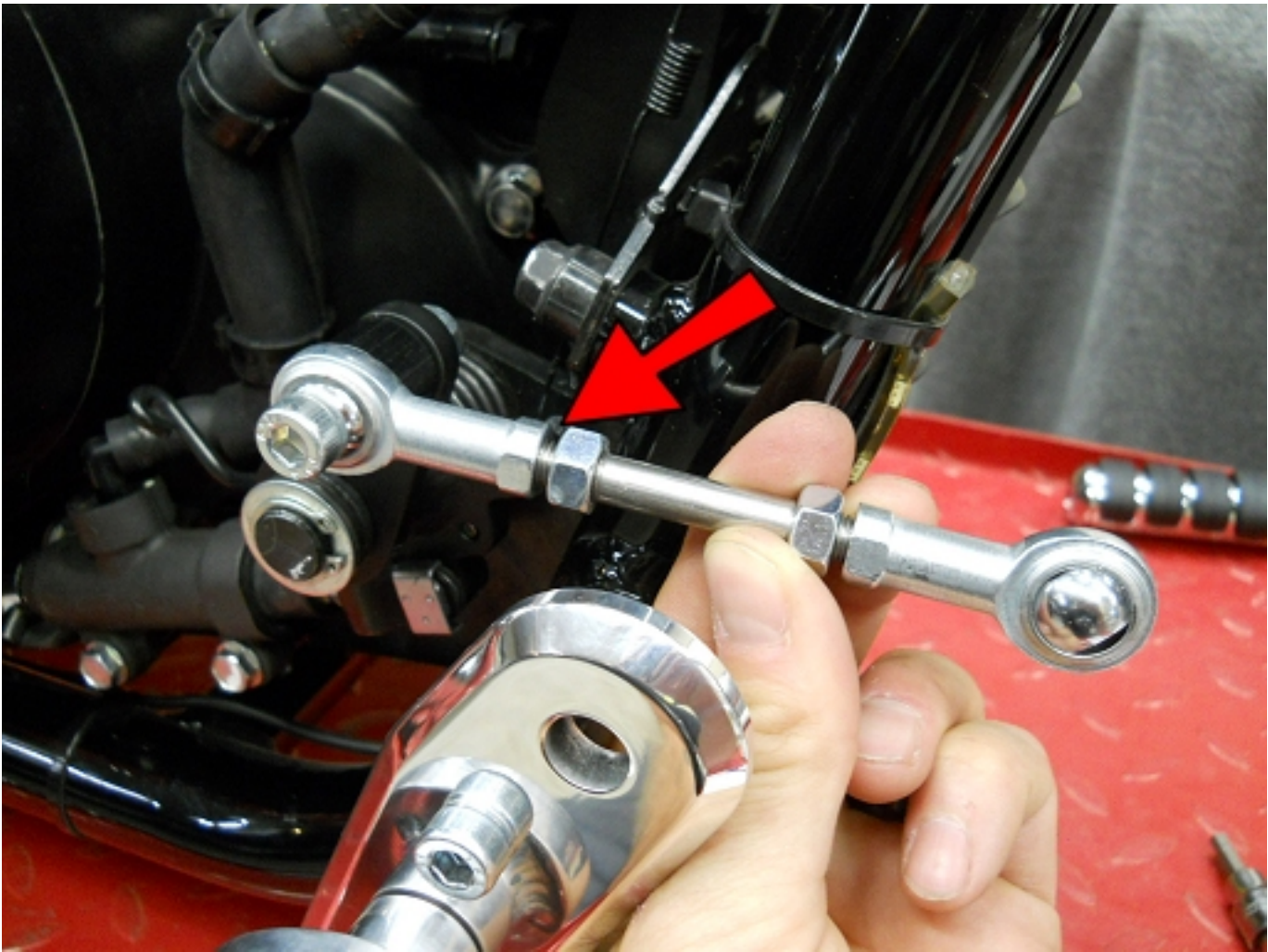
Thread the other end into the Rod End already on the ARM18.
