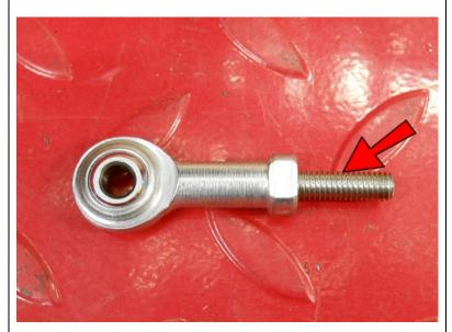
Thread an M6-1.0x40 Stud almost half way into an M6 Spherical Rod End.
