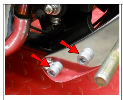
Secure the FC21 Plate through the brake master cylinder mount and to the frame.
