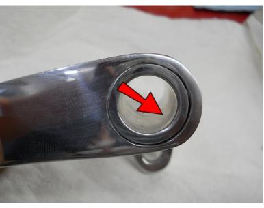
The inside of the Brake Pedal will likely have some polishing compound residue. Use a cloth or paper towel and make sure the inside is ABSOLUTELY clean. This will affect how well your Brake Pedal will rotate. After cleaning, put a little grease in there.
