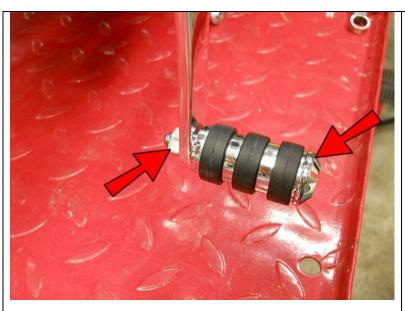
Install the Shifter Toe Peg and secure with a 5/16-24 Nut.
