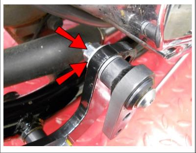
Connect to the top hole of the STOF8, clean any excess grease off of the bolt and secure with a 5/16" Washer and a 3/8-16 Nut.
