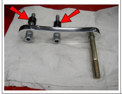
Place a 1/2" Spacer onto both of the M10-1.25x70 Socket Head Bolts.
