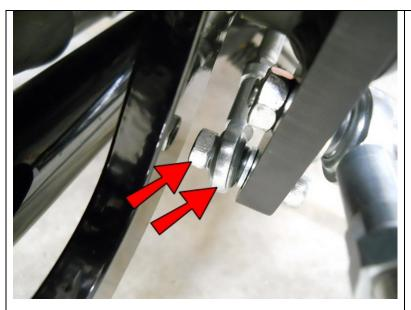
Pull the M6-1.0x25 Socket Head Bolt back out just enough to give you room to place the end of the original linkage onto the bolt and secure with an M6 Nut. Note: Make sure the M6 Washer does not fall off when you are doing this.
