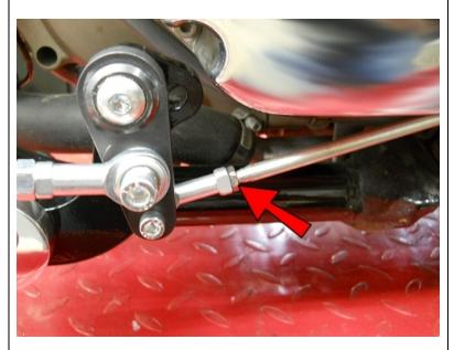
Adjust the Shifter Pedal height with the original linkage. Make sure there is enough thread in both ends for a secure connection. If you need more adjustment, you can remove the front linkage from the Pedal and adjust it as well, then reconnect. After the height is adjusted to the desired position, tighten the nuts against ALL of the Spherical Rod Ends.
