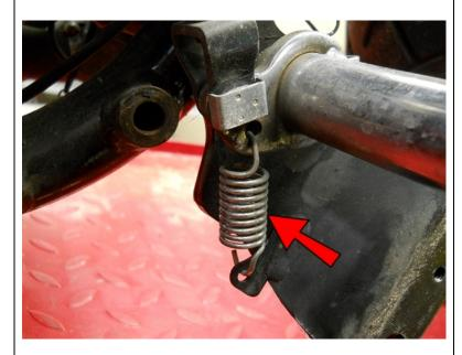
Using needle nose pliers, remove the bottom hook and then the top hook of the brake return spring.
