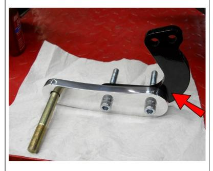
Place the STOF8 onto the two M10-1.25x70 Socket Head Bolts.
