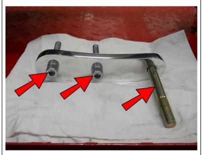
Insert two M10-1.25x70 Socket Head Bolts and a 1/2-20x4 Hex Head Bolt into an FC21 Plate as shown.
