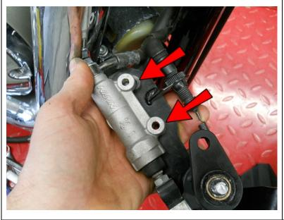
Hold the entire assembly flat in your hand to make it easier to replace the spacers between the master cylinder and it's mount and line up the holes.
