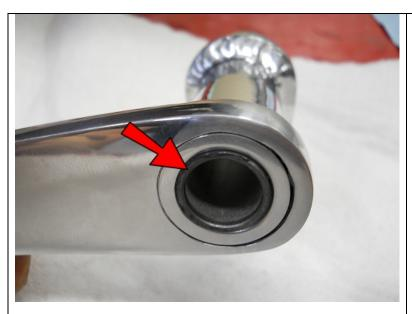
Place two SLV4's into the Brake Pedal.
