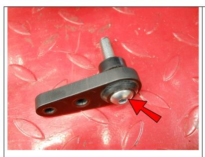
Insert a 3/8-16x2.25 Button Head Bolt into the ARM20 that you previously installed the sleeves into.
