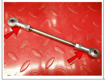
Then thread on 5/16" Spherical Rod Ends.
