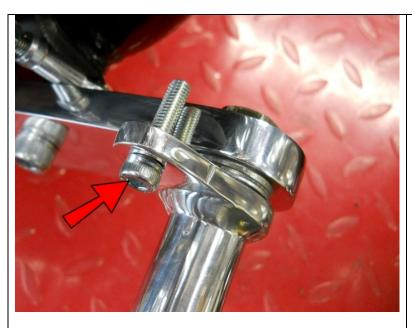
Insert an M6-1.0x25 Socket Head Bolt into the Brake Pedal.
