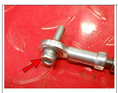
Insert an M6-1.0x25 Socket Head Bolt into one of the M6 Spherical Rod Ends.
