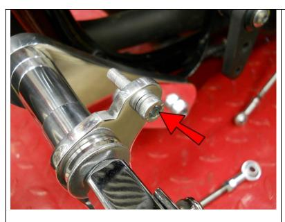
Insert an M6-1.0x25 Socket Head Bolt into the Shifter Pedal.
