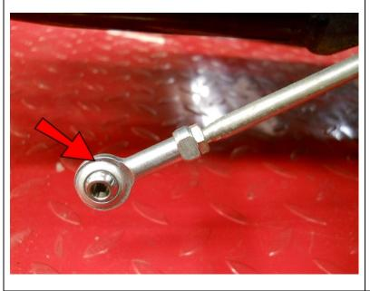
Thread the original shifter linkage back into the shifter arm on the spline where you removed it from. (Left Hand End). Now Thread an M6 Spherical Rod End onto the other end as shown.
