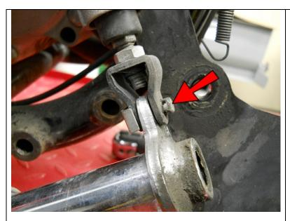
Remove this clevis pin to remove the brake pedal.
