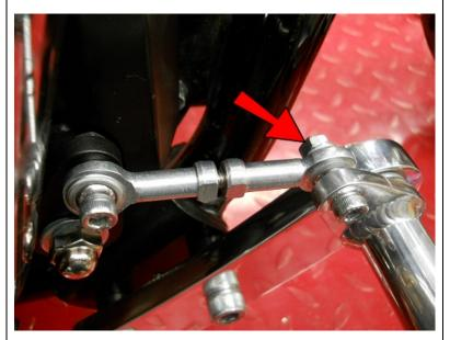
Thread an M6 Nut on and just tighten enough to snug it at this point. Do not use threadlock here yet. (You ARE using threadlock right?)
