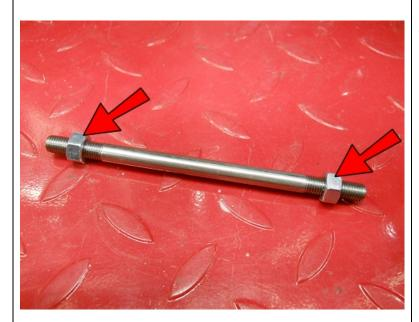
Thread 5/16-24 Nuts about half way onto both ends of the supplied Shifter Linkage.
