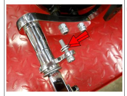
Place TWO M6 Washers onto the bolt.
