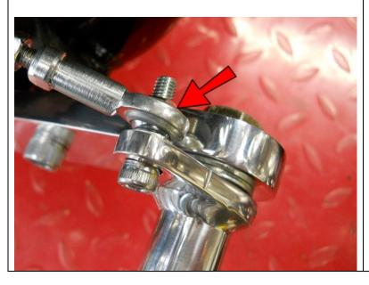
Place the other end of the Linkage onto the M6-1.0x25 Socket Head Bolt.
