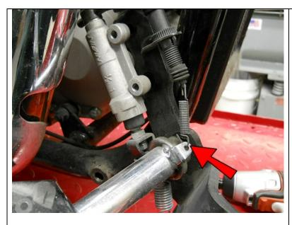
Unhook just the bottom hook of the brake switch spring.
