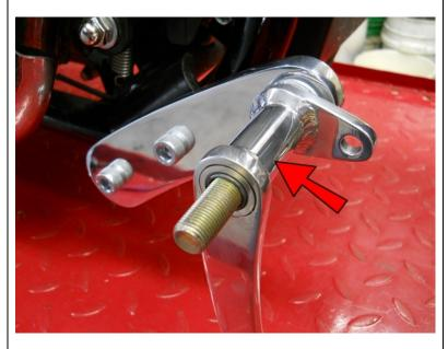
Slide the Brake Pedal onto the 1/2-20x4 Hex Head Bolt.
