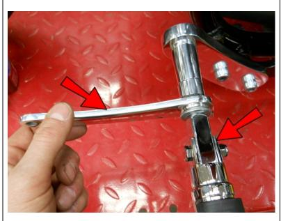
Install a foot peg and tighten. Then make sure the Shifter Pedal rotates freely. If it does not, stop now and correct.
