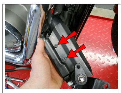
Replace the heat shield and secure with the bolts removed earlier.
