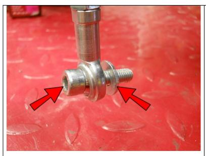
Insert an M8-1.25x30 Socket Head Bolt into the other end of the linkage then slide a 1/4" Washer onto the bolt.
