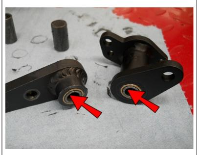
Now, insert 2 of the SLV1 into the ARM21and the other one into the ARM20.
