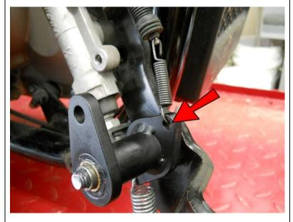
Place the bottom hook of the brake switch spring into this hole of the ARM21.
