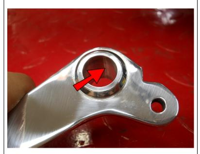
Clean the Shifter Pedal as you did with the brake side and grease.
