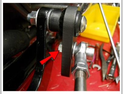
Connect to the middle hole of the ARM20 and secure with an M8 Nut.
