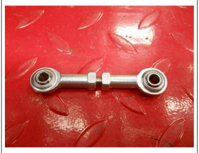
Thread another M6 Spherical Rod End almost all of the way onto the other end of the M6-1.0x40 Stud.
