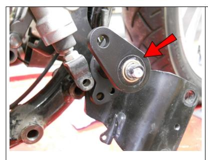
Place the ARM21onto the 3/8x3 Hex Head Bolt as shown. Clean any excess grease off of the bolt.
