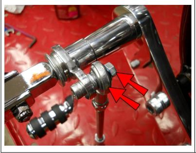
Place one end of the Shifter Linkage onto the bolt and secure with an M6 Nut.
