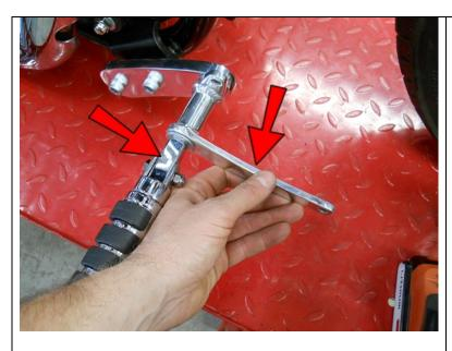
Install a foot peg and tighten. Then make sure the brake pedal rotates freely. If it does not, stop now and figure out why. Note: You should not have to make the foot peg loose for the Pedal to rotate correctly.
