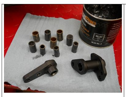
Apply some axle grease to all of the SLV1, SLV4, Bronze Sleeves, ARM20 and ARM21.
