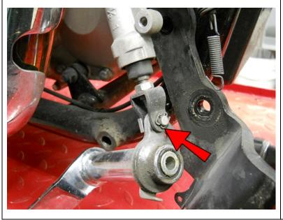
Turn the brake pedal so that you can get to this cotter pin. Cut and remove it.
