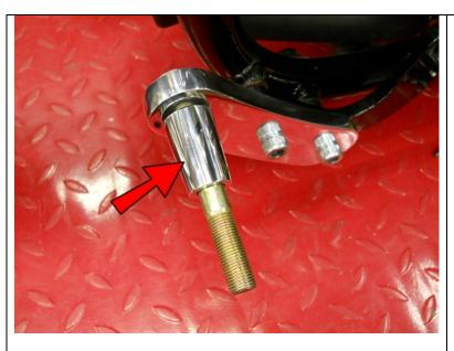
Secure the assembly to the frame and slide a STOF4 on as shown.
