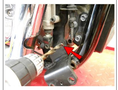
Drill this hole a little bigger using a 3/8" drill bit.
