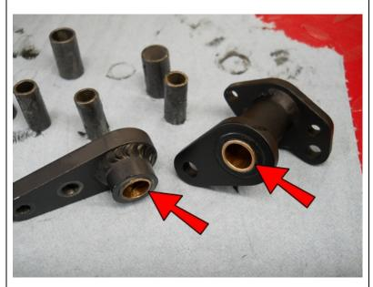
Insert 2 of the Bronze Sleeves into the ARM21and the other one into the ARM20.
