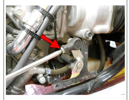
Loosen this nut and thread it the rest of the way onto the linkage rod. (It is a LEFT HAND thread.)
