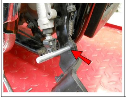
Place the 3/8x3 Hex Head Bolt into the hole from the back.
