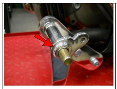
Place the Shifter Pedal onto the bolt.
