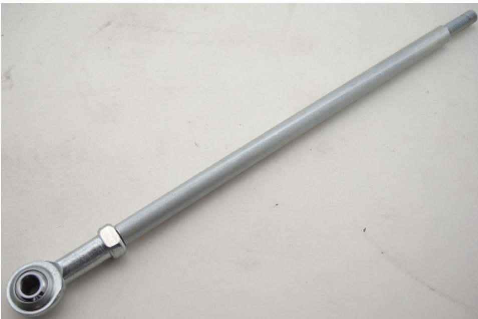
Thread a Spherical Rod End onto the shift linkage.
