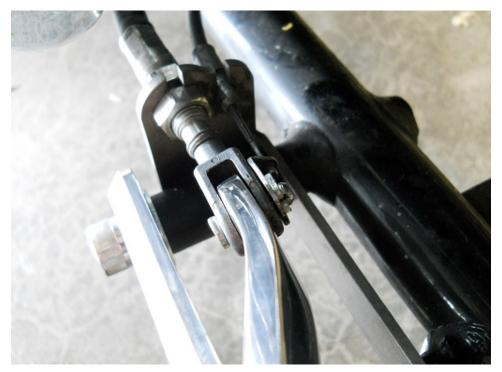
Orient the Brake Linkage with the spring hole end toward the back and attach to the brake cable and brake light switch cable with the clevis pin that you removed previously and a new Cotter Pin.
