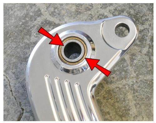
Prepare the Brake Pedal and Shifter Pedal by applying grease to the outside surface of the SLV1's and the inside and outside of the 5/8x1/2 Bronze Sleeves. Place the SLV1's into the 5/8x1/2 Bronze Sleeves and insert them into the Brake Pedal and Shifter Pedal. Install a Toe Peg into the end hole of the Brake Pedal and Shifter pedal and secure with a 5/16 Nut.
