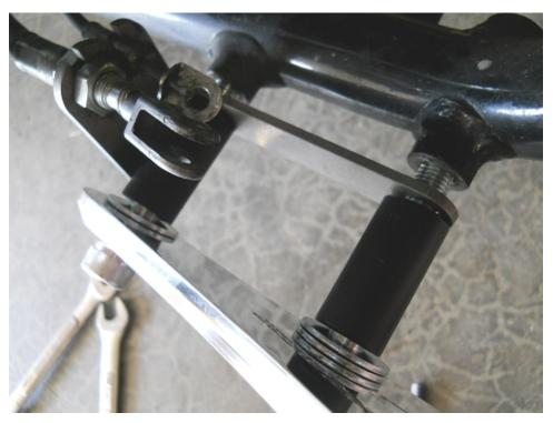
Insert an M10-1.25x70 bolt into the bottom holes of the FC6-R. Place one 3/8" Washer onto the back bolt and two 3/8" Washers onto the front bolt as shown. (If it looks like more washers, that's just a reflection.) Place the 1.5" Spacers onto the bolts, line the bolts up with the holes of the BSM2 and thread into the frame and tighten. You may need to work some slack in the cables to get it all to line up. This is why you previously loosened them.
