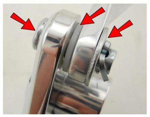
Attach the other end of the Brake Linkage to the Brake Pedal with a  $5/16 \times 7/8$  Clevis Pin, a 3/8" nylon washer, a 1/4" Zinc Washer and cotter pin as shown.
