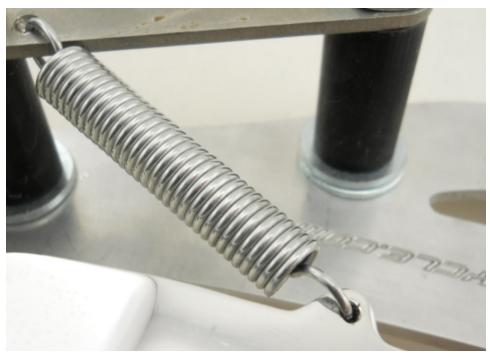
Hook one end of the spring into the small hole in the BSM2 and the other end of the spring into the small hole in the Brake Linkage.
