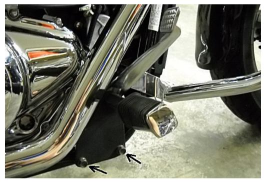
On the brake side, remove the stock foot control bracket by removing the two 10mm bolts attaching it to the frame.
