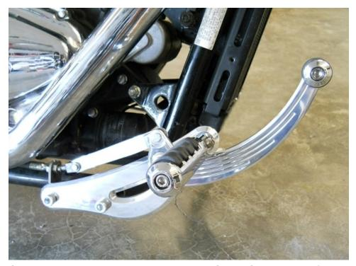
Connect the Brake Pedal to the outside of the FC6-R with a 3/8-16x2 Button Head Bolt and secure with a 3/8 nut.
