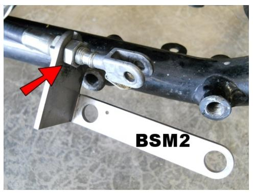
Insert the brake cable and brake light switch cable into the slots of the BSM2 in the same manor you removed them but only finger tighten the nuts, so that you can adjust the linkage slack after connecting the Brake Pedal.
