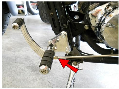
Tighten the M6 Nut against the Spherical Rod End on the Linkage.
