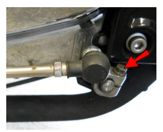
You may find the shifter pedal to be too low or high. If so, adjust as follows. Remove the bolt from the rear shifter arm and remove the arm from the spline. Rotate the arm one way or the other a couple notches to desired position and reconnect.
