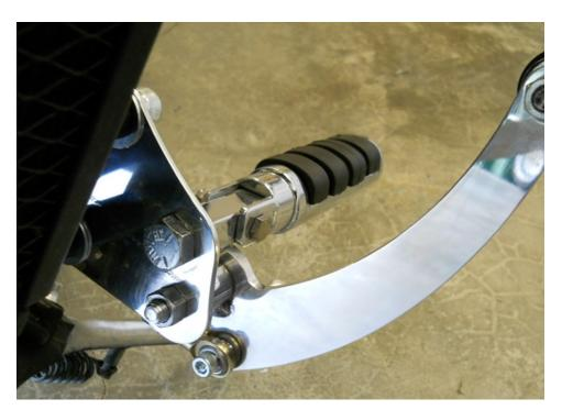
Install a foot peg into the top hole of the FC6-L. Connect the Shifter Pedal to the outside of the FC6-L with a 3/8-16x2 Button Head Bolt and secure with a 3/8 nut. Attach the other end of the Shifter Linkage to the Pedal with an M6-1.0x25 Bolt and secure with an M6 Acorn Nut on the front.
