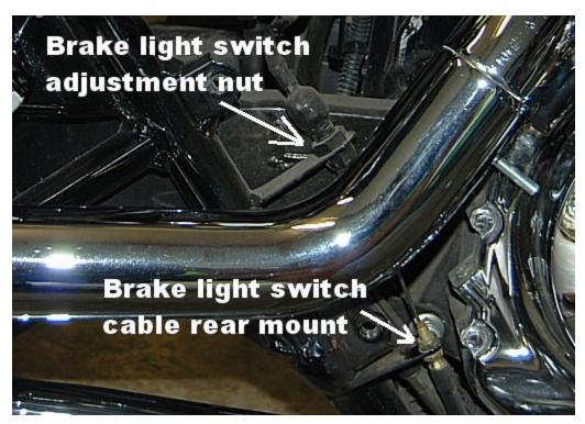
Remove the 3 bolts holding the upper and lower right side covers and remove the side covers. This can be done without removing the exhaust if you carefully work the cover out from behind it. Turn the brake light switch adjustment nut all the way counterclockwise to create slack in the cable. Loosen the top nut on the brake light switch cable rear mount.
