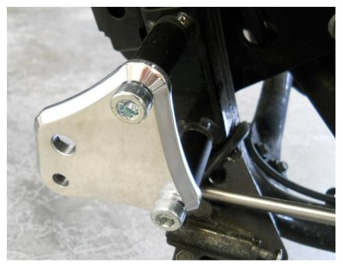
Attach the FC6-L to the frame with the M10 bolts, washers and spacers as before, BUT, only use one washer on each bolt, on this side.
