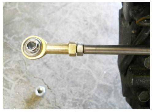
Thread the supplied M6 Nut and Spherical Rod End onto the other end of the Linkage but do not tighten them yet.
