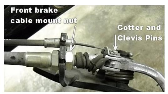
Remove the brake cable and brake light switch cable from the brake pedal by removing the cotter pin and clevis pin connecting it. Loosen the nut on the front brake cable mount all the way and slide it forward so that there is enough cable exposed to remove the brake cable through the top slot on the brake cable mount. Also remove the brake light switch cable.
