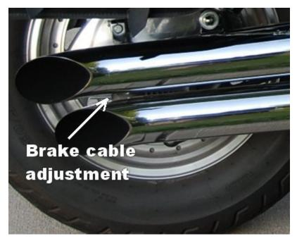
At the rear brake drum loosen the adjusting nut on the brake arm to allow plenty of slack in the brake cable.
