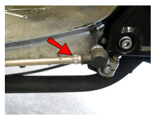
Remove the shifter linkage by loosening the nuts on both ends and rotate the linkage until it comes out of the ball joint on the shifter arm and the shifter pedal. Thread the right hand threaded nut from the old shifter linkage onto one end of the new Shifter Linkage. Now thread the Linkage into the ball joint on the stock rear shifter arm and tighten the nut against the ball joint.
